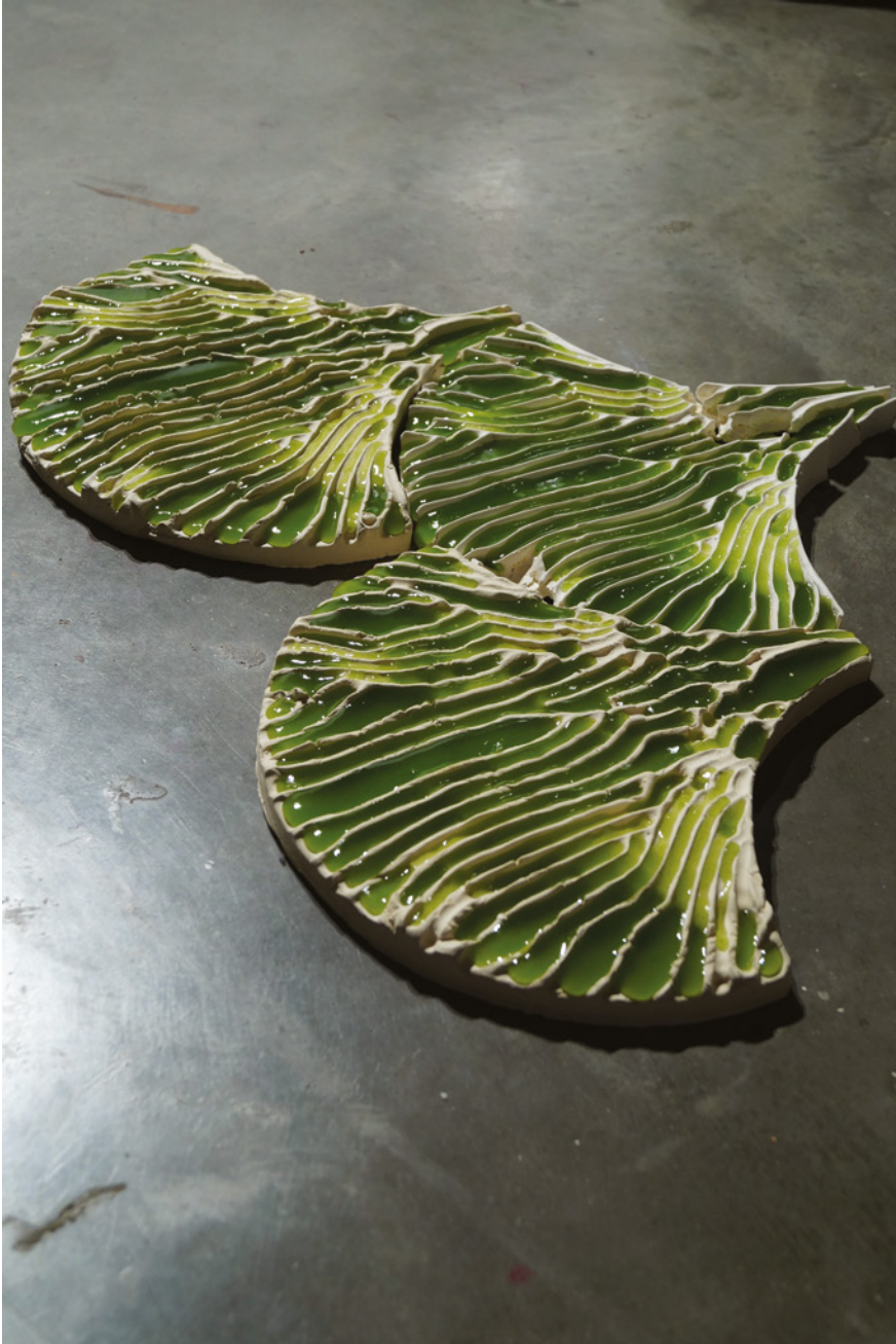
FIGURE 11.5 INDUS 1.0 – ceramic tiles with extruded algae-laden hydrogel, 2018–19. Team: Shneel Bhayana, Brenda Parker, Marcos Cruz and the Bio-Integrated Design Lab at UCL
