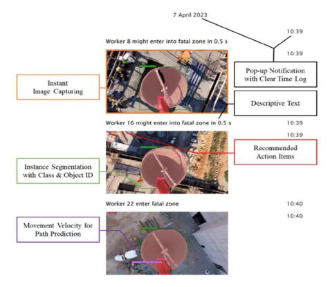
Figure 6: Demonstration of predictive warning mechanism in video processing
