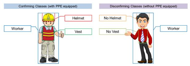
Figure 3: Definition of PPE statuses of a worker
