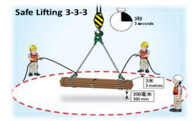
Figure 5: Definition of Safe Lifting 3-3-3 Principles
