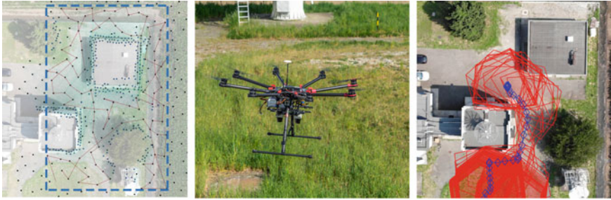
Fig. 3 In the middle the DJI drone used for the experiments. On the right the experimental test of the mt-MPC approach. Closed-loop trajectory obtained with mt-MPC (blue line with ‘ \diamond ’). Safe set \mathcal{X}(k) at different time step k in red. On the left the reachability graph obtained with G-BEAM without providing an external target
