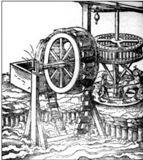
Fig. 47: A “Paternosterwerk” drawing water, set in motion by a horse mill. Woodcut by Peter Flotner, after: Walter Hermann Ryff, “Vitruvius Teutsch”, Nuremberg: Johan Petreius 1548, p. 304.
