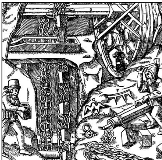
Fig. 45: A “Paternosterwerk” with chains and scoops attached to them, moving on a shaft on which a treadmill was fixed, after: Agricola 1928, p. 145.
