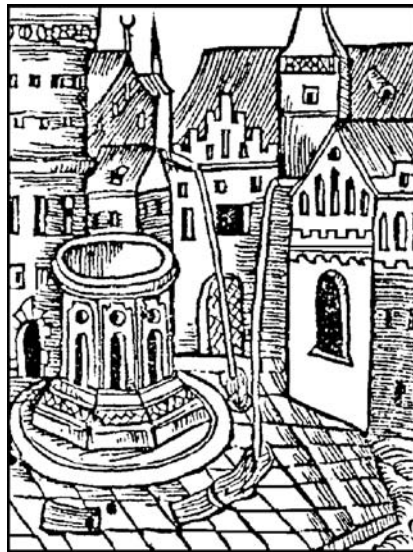
Fig. 19: Conducting water through gutters to public cisterns in town, after: Crescenzi-Trzycieski 1549, p. 32.
