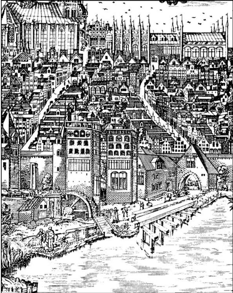
Fig. 52: Lübeck. A fragment of a woodcut by Elias Diebel dating from 1552, with a wheel next to one of the two water towers for the networks: Brauwasserkunst and Kaufleutewasserkunst. On the bank of the River Wakenitz a master fountain-builder with his helper manually drill a wooden pipe, after: Grabowski/Mührenberg 1994, p. 28.
