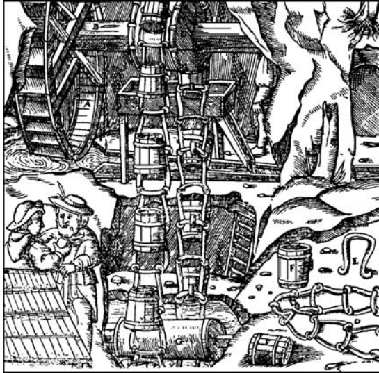
Fig. 46: A “Paternosterwerk” set in motion by a wheel powered by water from a stream conducted to a mine, after: Agricola G., 1928, p. 146.
