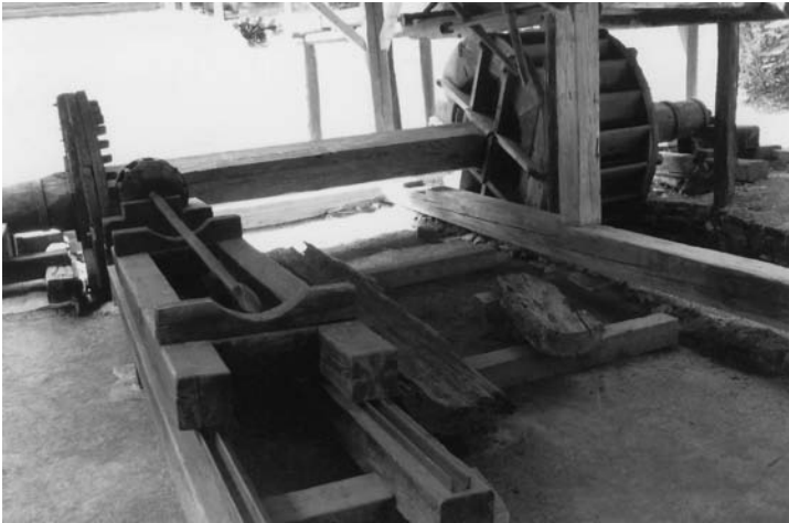
Fig. 58: A device dating from 1734 with a waterwheel for drilling wooden water supply pipes with a spoon auger. Bardejovské Kúpele (Slovakia), open-air museum. Photograph: B. Szurowa.
