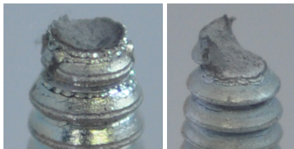
Figure 4-22 Tensile tests: Photos of failure modes of 6 mm carbon steel nails.
