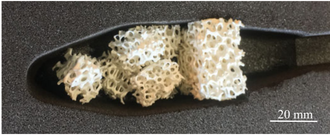
Fig. 33.24 Diced CFF ( 16 \times 16 \times 20\text{mm}^3 ) placed in a sand mold where a CFF with the dimensions of 35 \times 35 \times 20\text{mm}^3 keeps the dices in place
