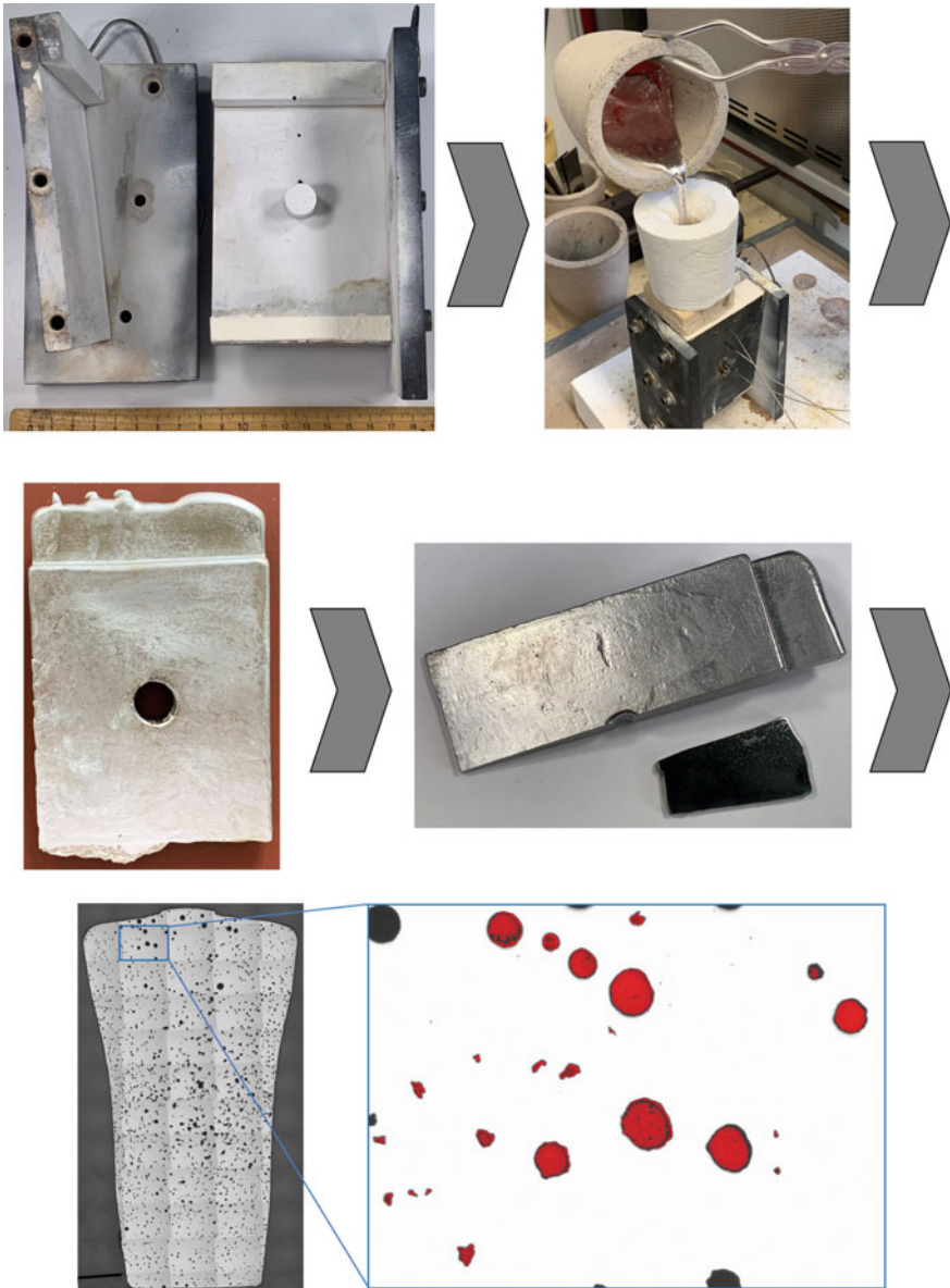
Fig. 9.11 Casting and experimental procedure for the determination of the pore size distribution
