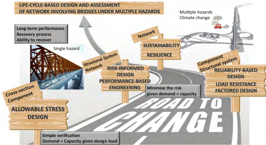
Fig. 7. Progress of structural design methodology: from the classical allowable stress design method toward the life-cycle based design and assessment of network involving bridges under multiple hazards.
