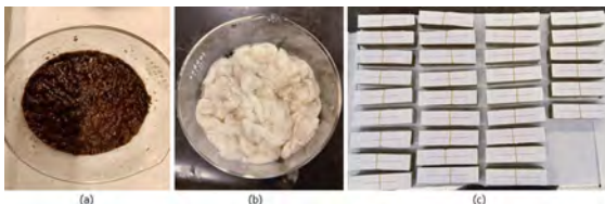
Fig. 1. (a) Type I-textile fibers; (b) Type II-textile fibers; (c) Textile-reinforced mortars after water curing.
