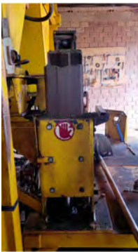
Fig. 8. Production of blocks using Ulva at a local company ‘SOIB’.
