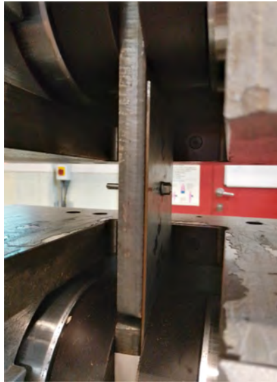
Fig. 4. Experiment of screwed connection (single-shear test method).
