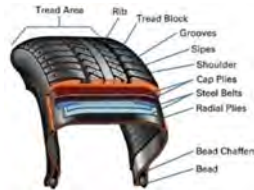
Fig. 1. Tire structure and engineered layers [23].
