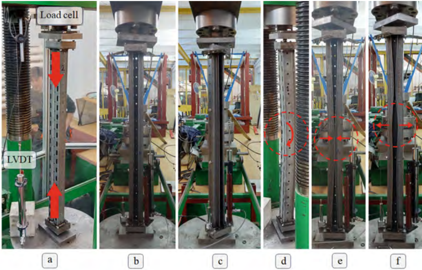
Fig. 4. Experimental tests: (a) non-reinforced specimen setup; (b) specimen setup for method 1 reinforcement with 2L-shaped profiles; (c) specimen setup for method 2 reinforcement with C-shaped reinforcement profile; (d) failure mechanism of the non-reinforced specimen; (e) failure mechanism of the specimens with 2L-shaped reinforcements; (f) failure mechanism of the specimens with C-shaped reinforcement.
