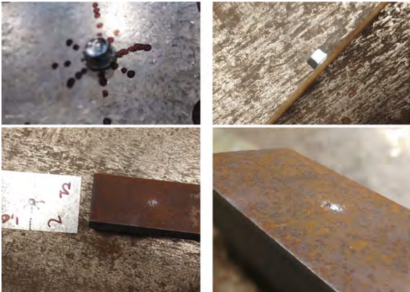
Fig. 8. Failed connection after test.
