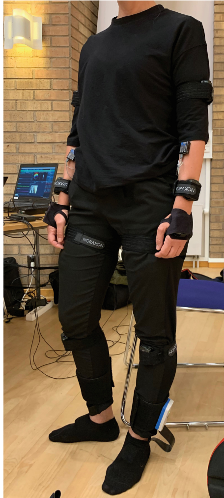
Fig. 3. Wireless EMG and motion sensor setup.
