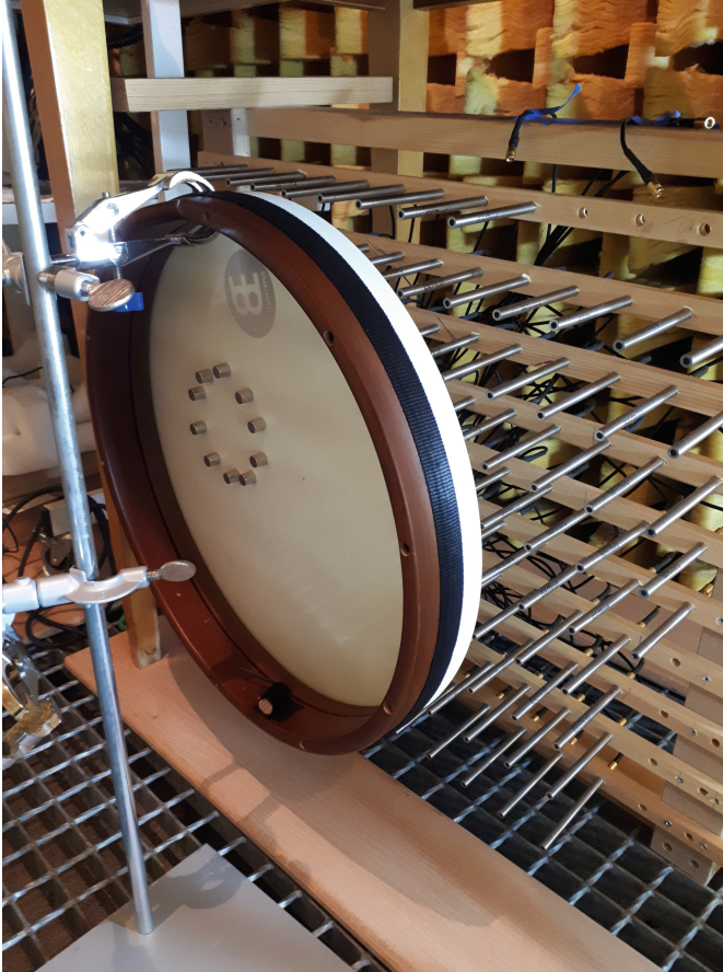
Fig. 2. Modified frame drum positioned in front of the microphone array.
