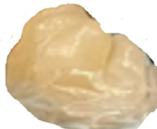
Fig. 6. Solidified brain tumor phantom with size of 5 cm.
