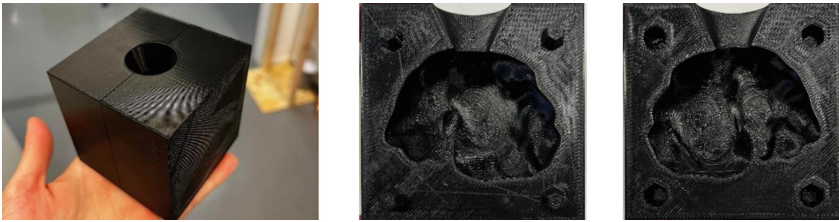
Fig. 5. 3D printed tumor molds.
