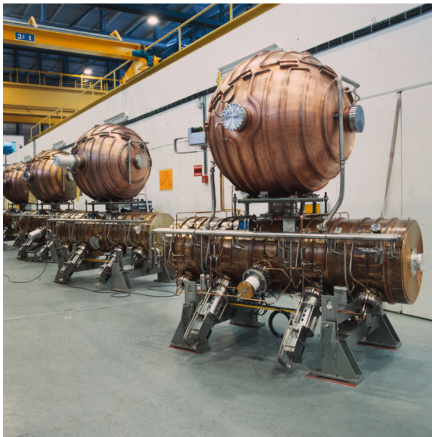
Fig. 10.5 The spherical storage structure on top of LEP's copper accelerating cavities saved energy by ensuring that the accelerating field was applied only when beams were passing through the accelerating structures and stored at other times (©CERN, All rights reserved).
