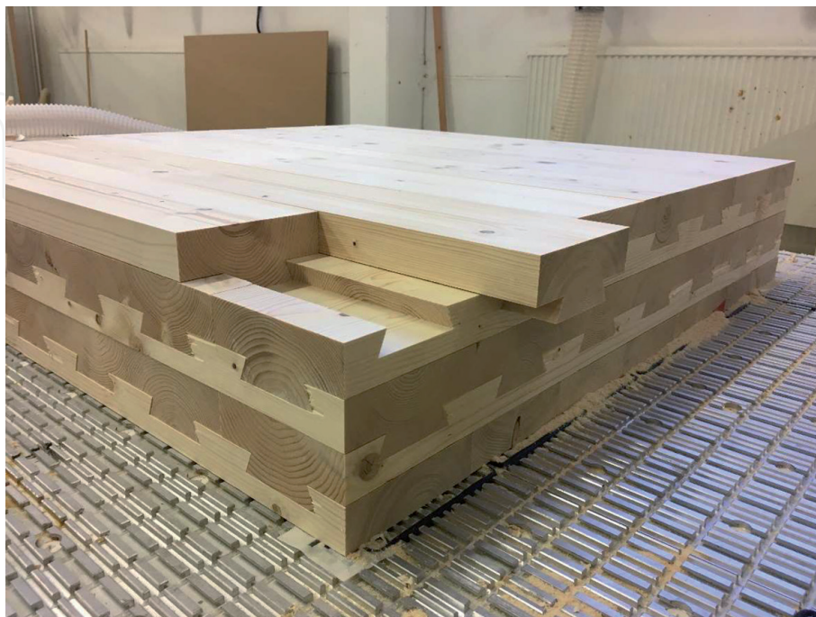
Figure 4. Adhesive- and metal fastener-free dovetail wood board element.
