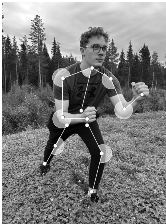
Figure 12.1 Kinect-based angle calculations are made by looking at the human body's different angles. Photograph by Satu-Maarit Korte.
