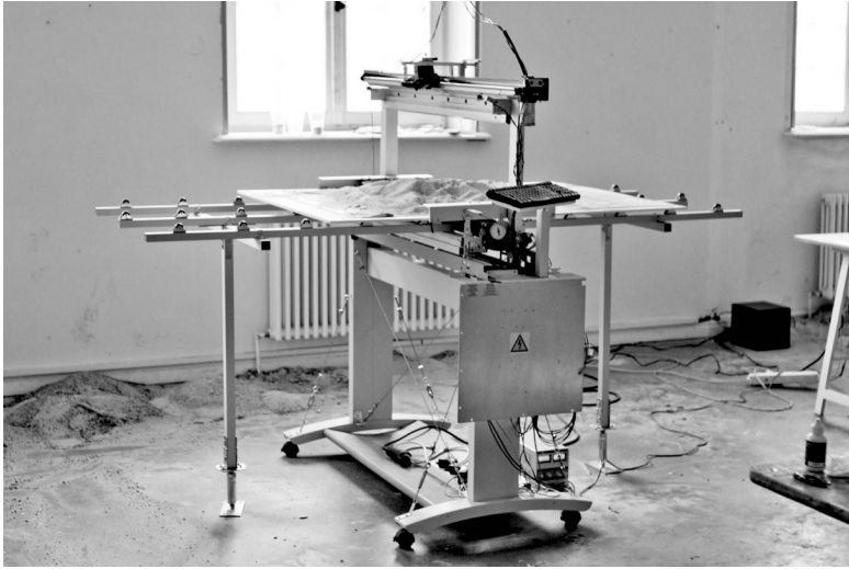
Plopper (Dual-Axis Precision Deposition System), CNC machine, hacked plotter, custom software and gcode, 4' × 7' × 5', Stuttgart, Akademie Schloss Solitude. 7
