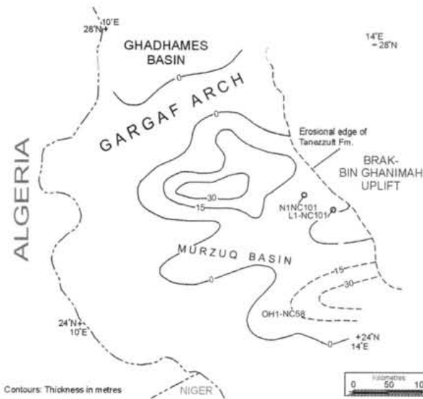
Fig. 5.3. Outline map of the Murzuq basin. The contours show the thickness of the Tanezzuft 'hot shale' (modified from Hallett 2002).
