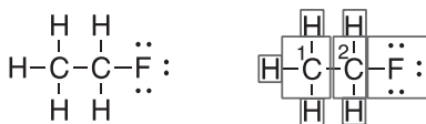
Figure 19.2 Ethyl fluoride (left) and ethyl fluoride with bonding electrons apportioned to the more electronegative atom (right).
