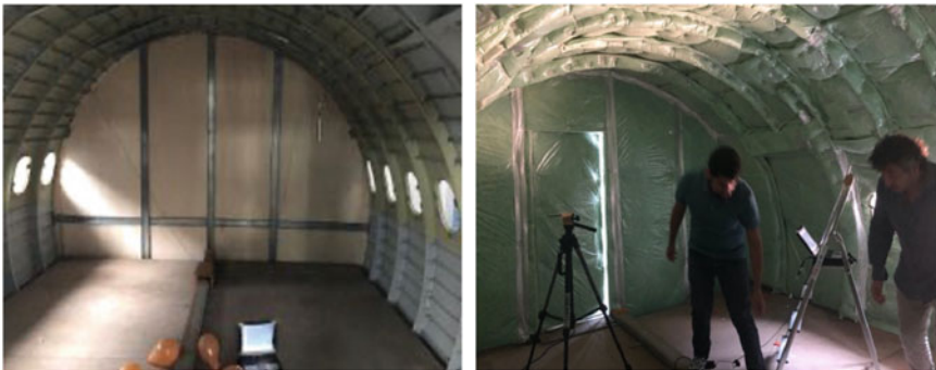
(b) Vibroacoustic tests of a fuselage bare structure (left), and of the furnished structure (right).
