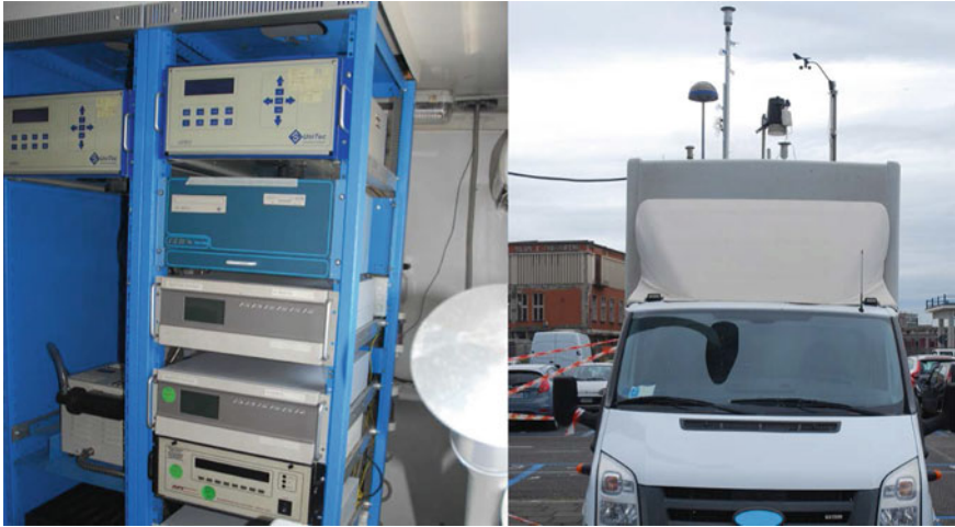
Fig. 4 The instrumentation used for revealing the contents of the air in port (left) and the equipped van with sensors (right)
