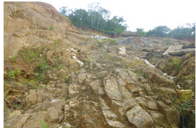
Fig. 5 Highly fragmented rock at the crown of the slide (Photo by Dias, A.A.V., July 2017)
