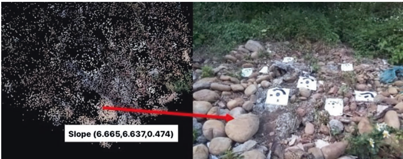
Fig. 13 Illustration of feature points in rocks at three-dimensional and two-dimensional image positions (initial position)
