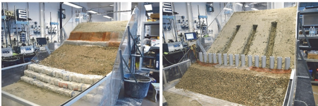
Fig. 42 Views at buttressing embankment behind the gabion wall in a silty slope and at pile wall, buttressing counterfort and excavated trenches in a clayey slope (Figs. 8g and 9e in Arbanas et al. 2023)
