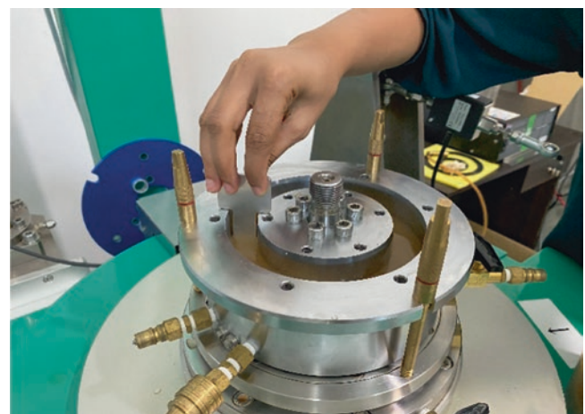
Fig. 5 Leveling the sample surface
