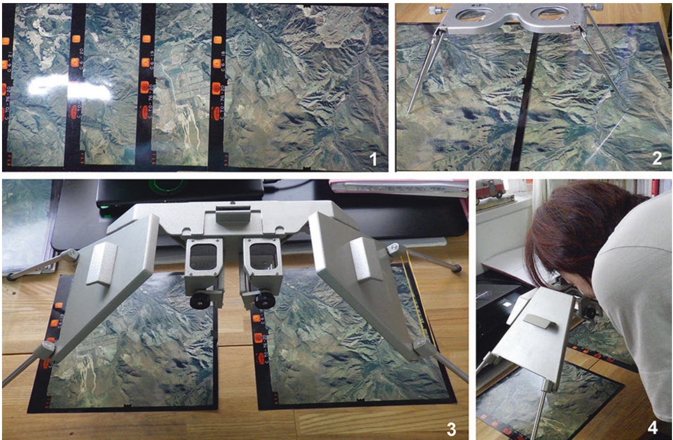
Fig. 14 Three-dimensional observation of aerial photographs of stereo pairs. 1. The close-contact print version of the aerial photograph describes the flight course, scale, shooting time, etc. 2. A photo of a simple stereo mirror and a stereo pair that can emphasize the undulations by about 2 times. 3, Reflective stereo mirror and photo. Pay atten-
