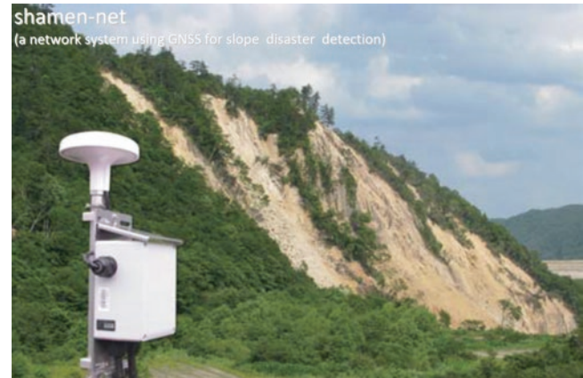
Fig. A.38 “Shamen-net” is a total monitoring system integrating GNSS and other monitoring device (Measurement precision: \pm mm, on a real time basis)
