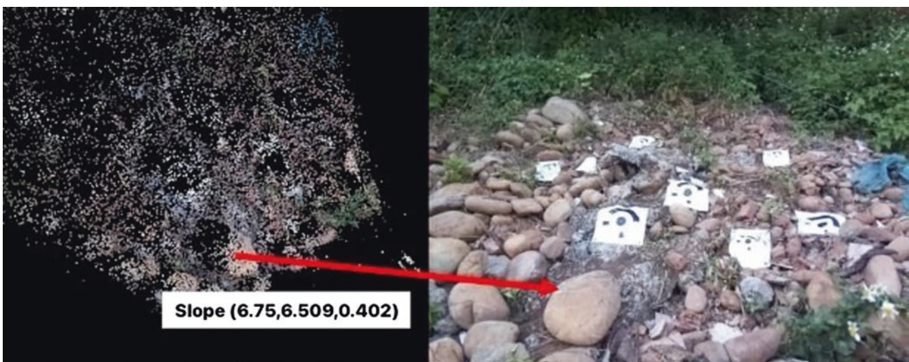
Fig. 14 Schematic diagram of feature points in rock at three-dimensional and two-dimensional image positions (15 cm movement)
