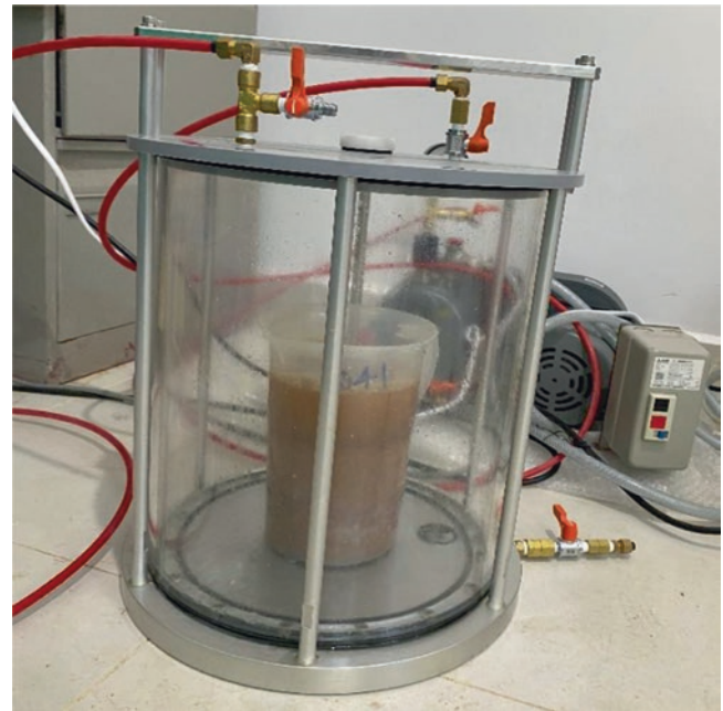
Fig. 4 De-airing the soil sample
