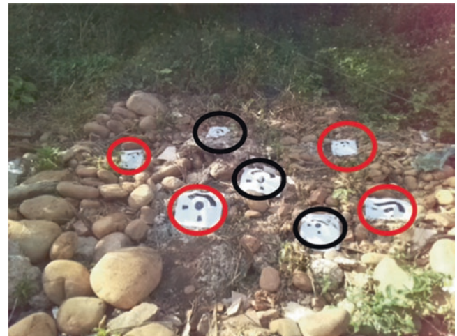
Fig. 9 Layout diagram of control points and checkpoints (red for control points, black for checkpoints)
