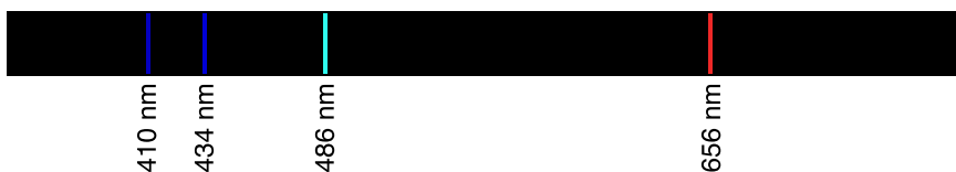
Figure 6.6 The atomic emission spectrum of hydrogen showing the spectral lines in the visible range and their corresponding wavelengths.
