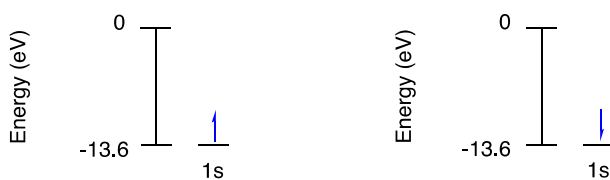
Figure 7.5 Energetically equivalent, ground-state electron energy diagrams for hydrogen with spin quantum number ( m_s ) +\frac{1}{2} (left) and -\frac{1}{2} (right).
