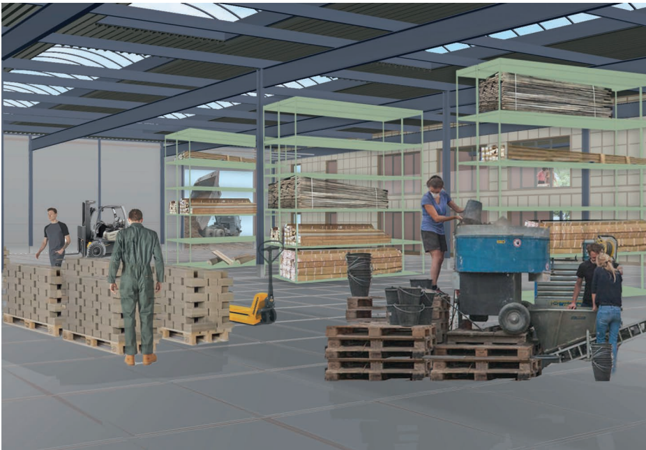
FIGURE 14.4 The Master's Design Studio 'Challenges to Metabolic Design' at the University of Ghent (2021) sought solutions to challenges of circular building, such as logistics issues. Gentiel Acar, Jesse Ghyssaert, Ferre Lust and Karen Steukers designed a multi-functional centre for the production, processing and sale of reclaimed materials. They designed the building from existing steel portal frames.
