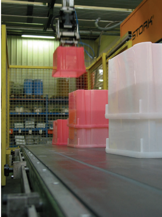
FIGURE 11.2 Example of industrial waste: colour transition in the production of plastic crates.
