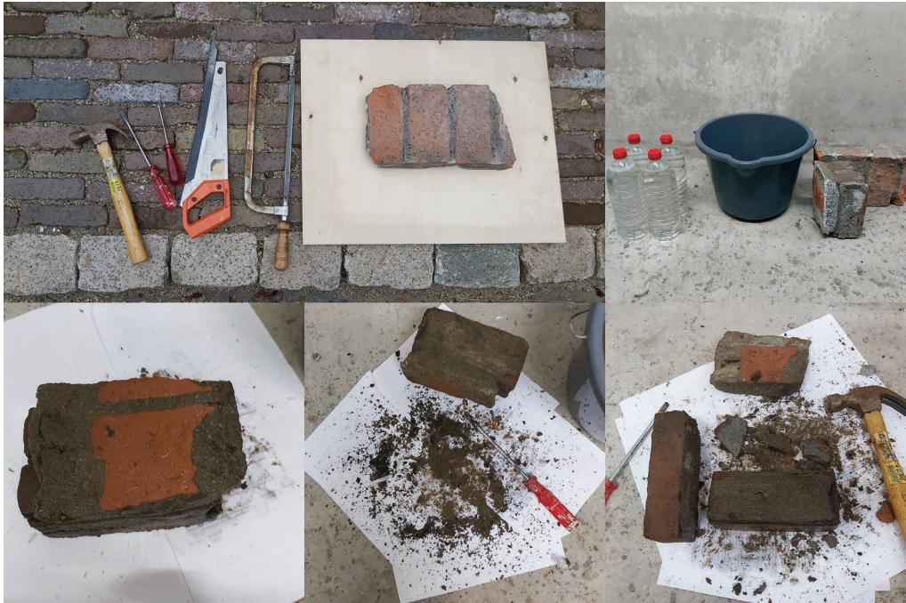
FIGURE 6.2 Separation of bricks using non-specialist tools, physical process experiment (days 2–5). Taking a lead from Ivan Illich’s philosophy described in Tools for Conviviality , 6 Derk Ringers responds to the challenge of manual disassembly of brickwork: “Bricks separated: 6/Amount of cleaning vinegar: 4 litres/Days soaking in vinegar: 3/Estimation of labour: 1.5 hrs”.
