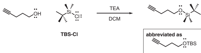
Figure 16.12 Use of a tert-butyldimethylsilyl (TBS) ether to protect the alcohol in pent-4-yn-1-ol.
