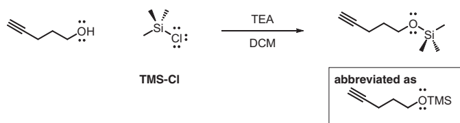
Figure 16.10 Use of a trimethylsilyl (TMS) ether to protect the alcohol in pent-4-yn-1-ol.
