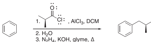
Figure 26.9 Friedel–Crafts acylation of benzene and Wolff–Kishner reduction, formally the attachment of a primary carbon atom to the ring.
