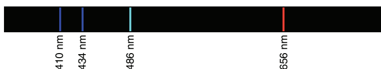
Figure 2.1 The atomic emission spectrum of hydrogen showing the spectral lines in the visible range and their corresponding wavelengths.
