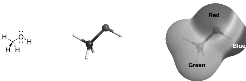
Figure 15.1 Structure ( left ), model ( middle ) and electrostatic potential map ( right ) of methanol (red corresponds to high electron density and blue corresponds to low electron density).
