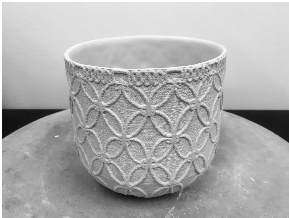
Figure 10.7 A cast cup revealing the trace of my freehand drawing, that of the digital fabrication of the mould making process, and that of the slip casting process. Photograph by the author.
