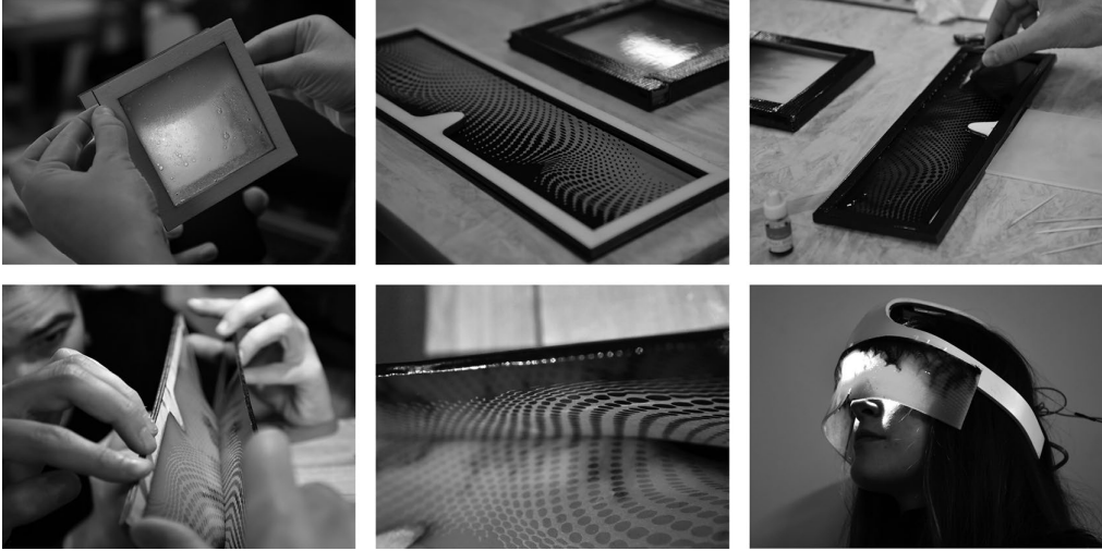
Figure 14.6 The methodology applied in a design workshop. Participants achieve personalized shapes and textures through laser-cutting and engraving on moulds, ultimately shaping a conceptual product prototype. Photographs by Laura Varisco.
