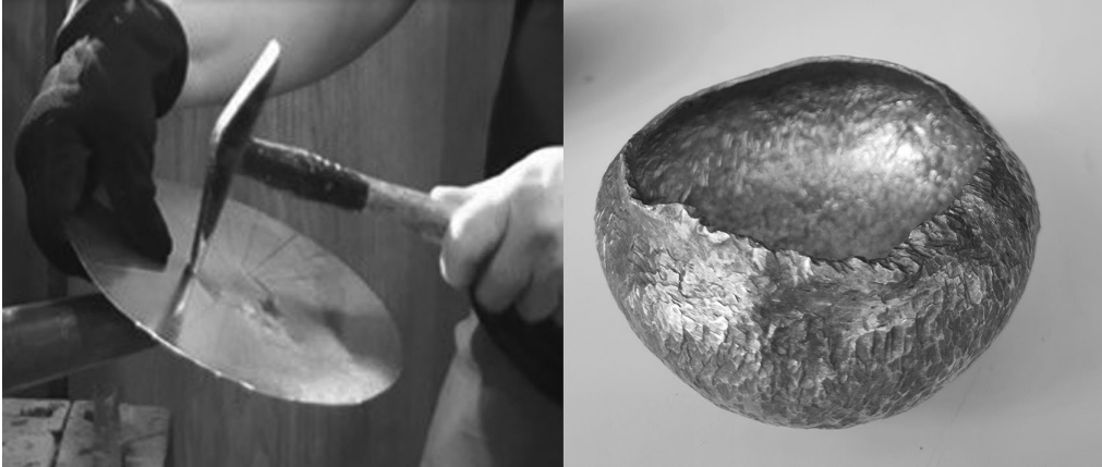
Figure 12.1 Working from metal sheet to a 3D form. Photographs by the author.
