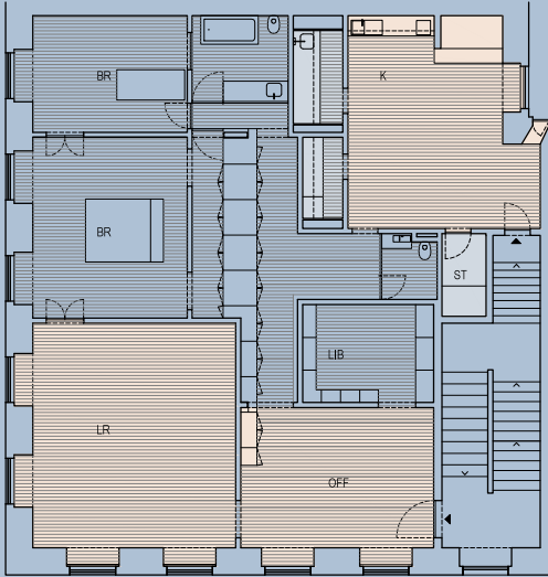
2nd floor Final plan after renovation
