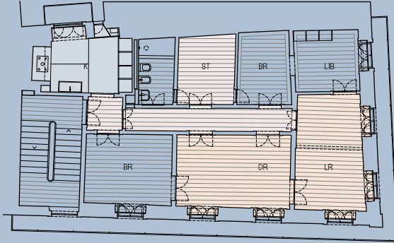
3rd floor Final plan after renovation
