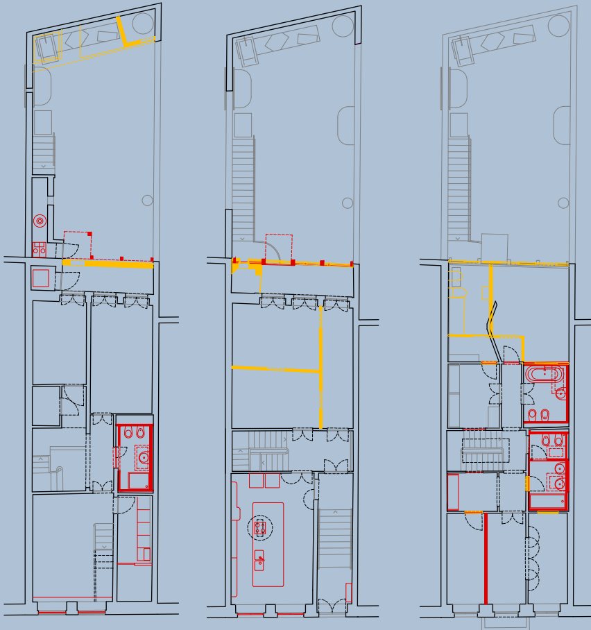
Lower ground floor | Ground floor | 1st floor 1:200 Changes introduced by the renovation project
