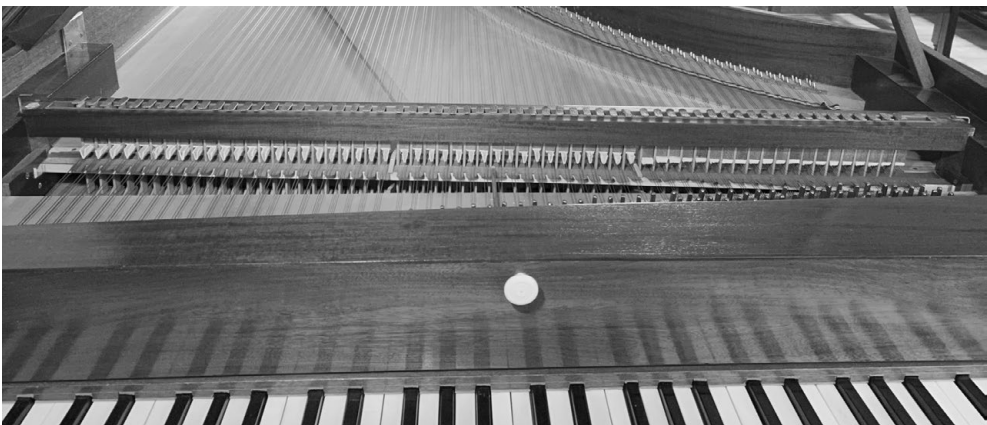
FIGURE 2 Above: Front view of the damper rail in a copy of a piano by Anton Walter, knee levers disengaged, all dampers lowered on the strings. Middle: Both sides of the damper rail raised. Below: Only the treble end of the damper rail raised. The changeover from damper wedges in the lower region to damper pads in the triple-strung treble is clearly visible.
