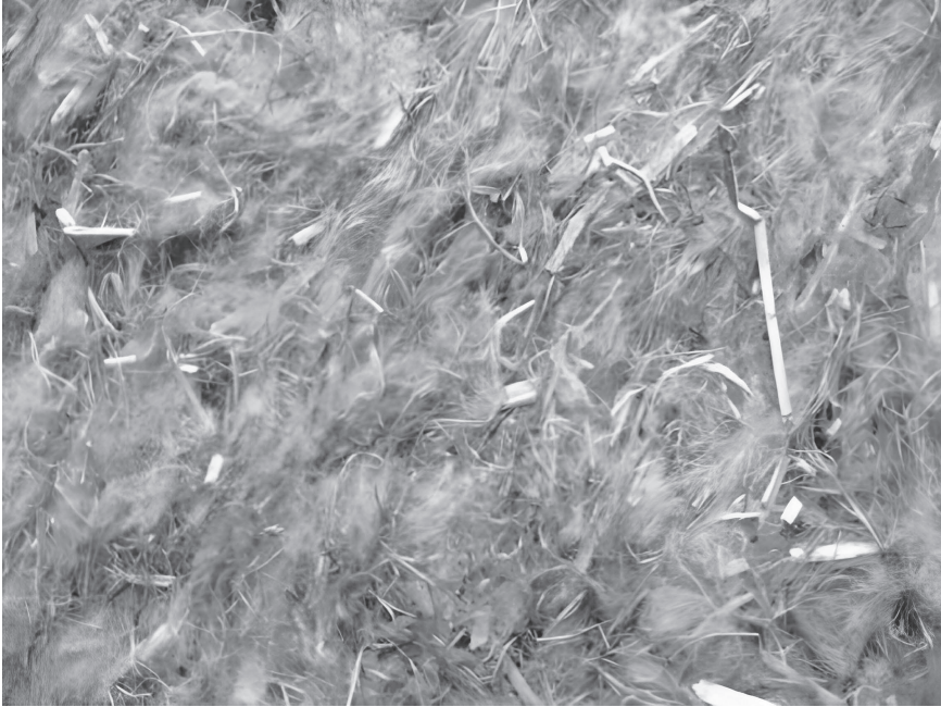
FIGURE 6.2 Detail of the structure of hemp. 5
