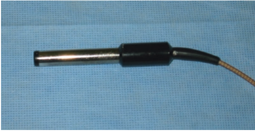
Fig. 16.5 The Kretztechnik 7200 solid probe is used for diagnostic standardized A-scanning and for biometry
