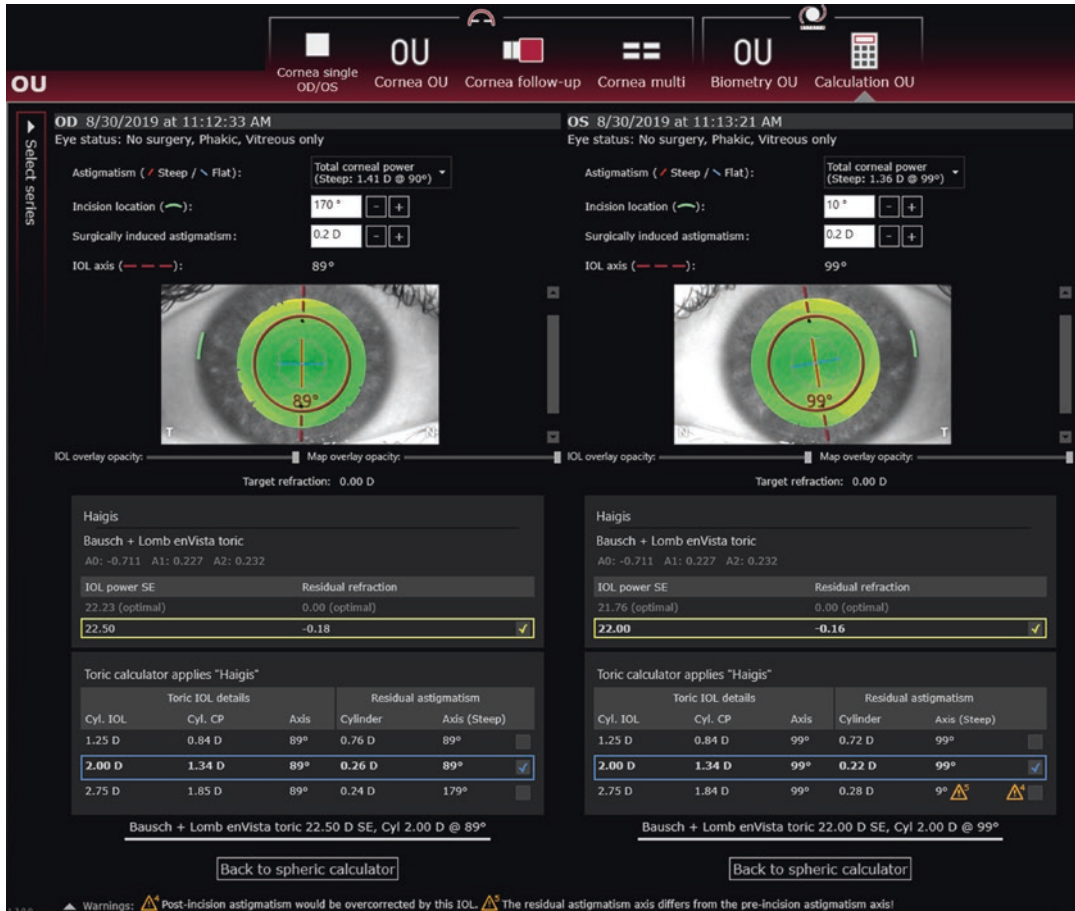
Fig. 22.5 ANTERION Cataract App: OU toric IOL calculator accounting for corneal astigmatism, incision location, and surgical-induced astigmatism
