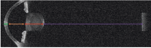
Fig. 19.1 Argos uses a segmented method to measure the AL using multiple indices of refraction. A specific refractive index is used for each segment, where: AL = CCT/1.375 + AD/1.336 + LT/1.41 + VIT/1.336 - RT
