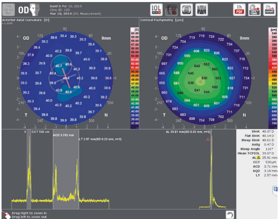
Fig. 27.7 Biometry display with interference curve, detected peak locations, indices, and selectable maps
