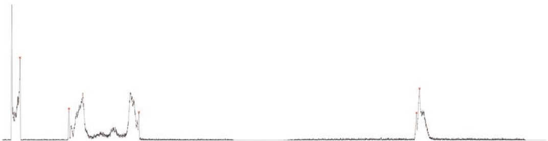
Fig. 11.2 Typical “A-scan” produced by an optical biometer. The first spike is the reflection produced by the air–corneal interface of the anterior cornea. The first “x” is above the spike produced at the posterior cornea. The second “x” is above the spike of the anterior capsule of the
