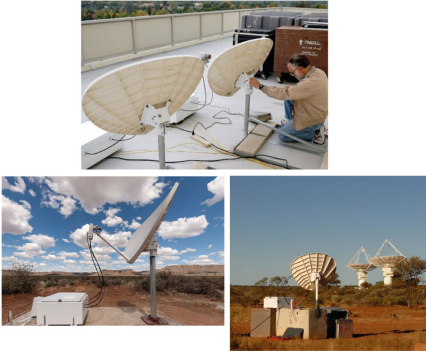
Fig. 8.4 (upper panel) Larry D’Addario adjusting a tropospheric monitoring antenna in a test installation on the roof of the Jet Propulsion Laboratory building in Pasadena, California, USA (credit: R.P. Millenaar, SPDO, 2010). (Lower left) One of the two elements of the tropospheric phase measurement interferometer deployed in the Karoo Desert, South Africa (credit: R.P. Millenaar, SPDO, 2011). (Lower right): One of the two elements of an identical interferometer deployed at Boolardy on Wajarri Yamaji Country in Western Australia (credit: R.P. Millenaar, SPDO, 2011)
