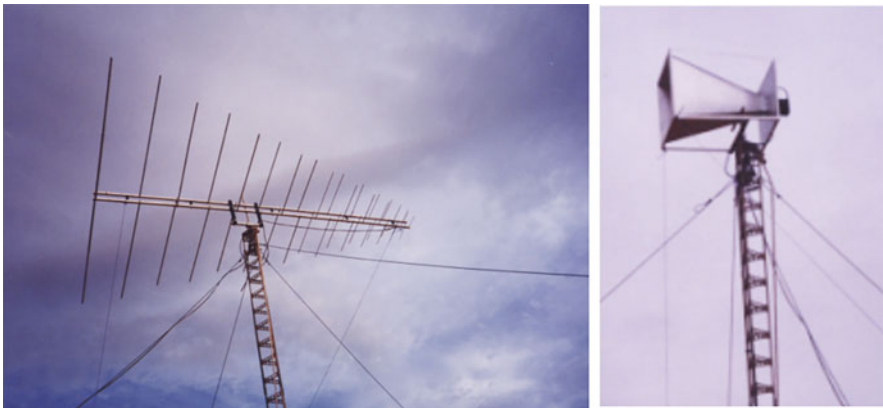
Fig. 7.3 left and right: Two of the antennas used to monitor RFI in the Murchison area of Western Australia in 2001 (Credit: Bruce Thomas, CSIRO Radio Astronomy Image Archive CRAIA-SKA003 (left) and CRAIA-SKA004 (right))
