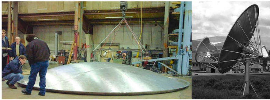
Fig. 6.14 Left: The first ATA reflector on the factory floor. Right: A completed antenna. Credit: David DeBoer
