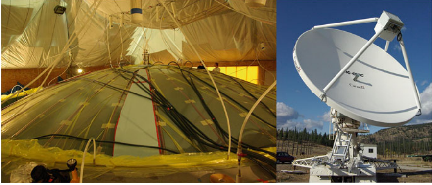
Fig. 6.11 Left: Vacuum Infusion of the 10-m Mk2 reflector at the Dominion Radio Astrophysical Observatory in Canada on June 4, 2008. Credit: National Research Council of Canada. Right: The reflector with the (PHAD) feed completed in October 2008. Credit: The National Research Council of Canada
