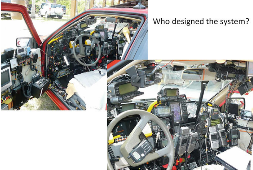
Fig. 6.3 An illustration of the complexity of stitching together devices which were developed with disparate interfaces and standards. Credit John T. McFarland
