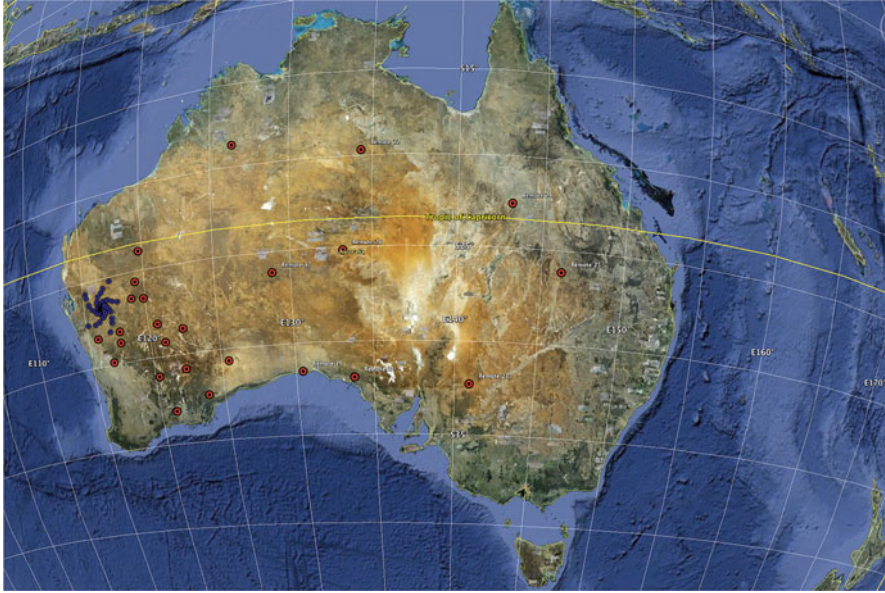
Fig. 8.5 The SKA array configuration proposed by Australia-New Zealand in 2011 in response to the Request for Information by the SKA Siting Group. The blue dots represent the core and mid regions of the array out to 180 km from the centre of the core, the red dots represent the locations of the remote stations provided in the A-NZ proposal. The white grid is 5 degrees on a side, corresponding to a fixed N-S length of 560 km and an E-W dimension (which varies with latitude) of 510 km along the Tropic of Capricorn (yellow line). (Credit: Fig. 6 in R. P. Millenaar, R. Bolton and J. Lazio, Array configurations for candidate SKA sites: design and analysis , 2011, report to the SSG and SSAC, hba.skao.int/SKAHB-481 )
