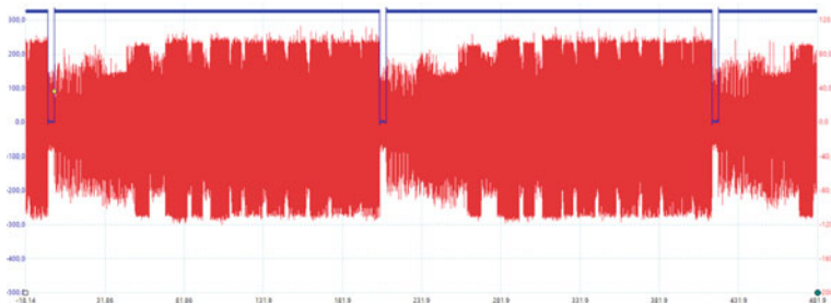
Fig. 4 An electromagnetic trace (red) of two consecutive inferences of a MobileNet (v2) model running on a Cortex M7 microcontroller. We can observe the clear separations between the convolutional basic blocks of the model. The blue line is a trigger signal showing the start and stop time sample of each inference
