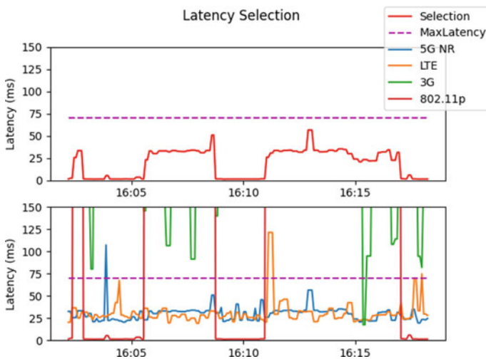
Fig. 10 Latency for the selected interface (top) and latency for all available interfaces (bottom)
