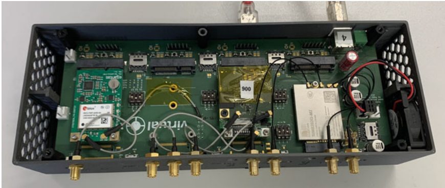
Fig. 3 The vehicleCAPTAIN development kit in Quad Expander configuration, with a Raspberry Pi 4 as the computing platform (underneath the circuit board). The Quad Expander configuration can host up to four mPCI-E or M.2 modules. The configuration is from left to right (i) Ublox F9P with 1pps, (ii) empty, (iii) Unex SOM301-E, and (iv) Simcom sim8202g
