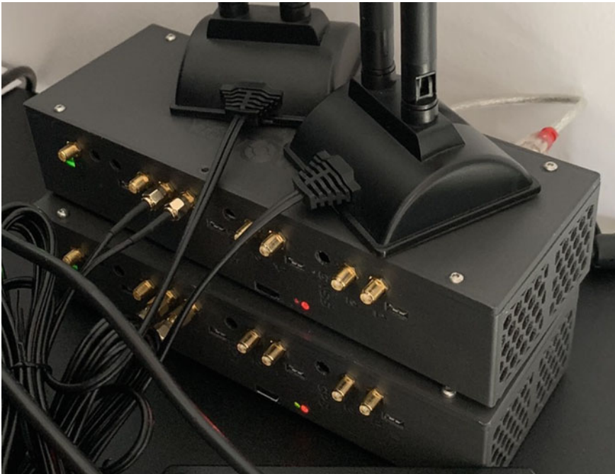
Fig. 6 Two vehicleCAPTAIN development kits stand on each other for continuous integration tests
