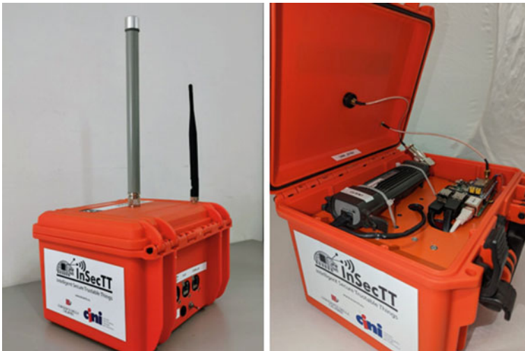
Fig. 12 Prototype of the forwarding device (FD) equipped with LoRa and Wi-Fi interfaces
