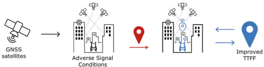
Fig. 9 Assisted GNSS or GPS improves TTFF in adverse signal conditions
