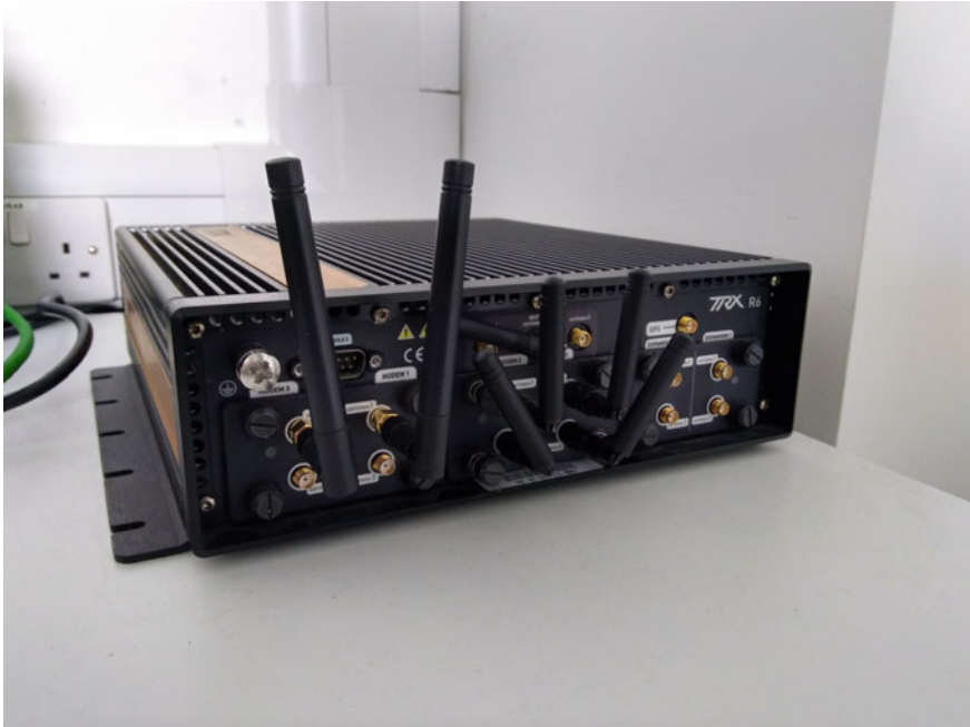
Fig. 1 KLAS TRX R6 with cellular modems. The expansion slot in the middle with the four short antennas contains the 5G modem. The left slot with the larger antennas contains modems for 3G and 4G
