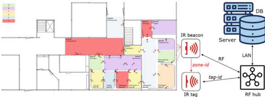
Fig. 6 IR tag-based localization solution
