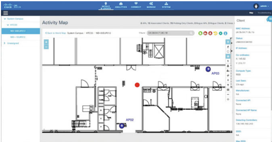
Fig. 4 Screenshot from CMX system showing the location of a Wi-Fi tag (red dot) and nearby APs (blue dots) in a test setup.
