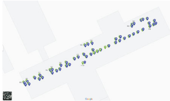
Fig. 5 Comparison of the two conversion methods from the local (metric) coordinates to GPS ones plotted on google maps. The green ones are calculated by the bilinear interpolation and the blue ones by ITMP
