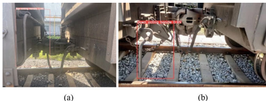
Fig. 8 Visualization of detection results. a Top acting handle detection results. b Down acting handle detection results
