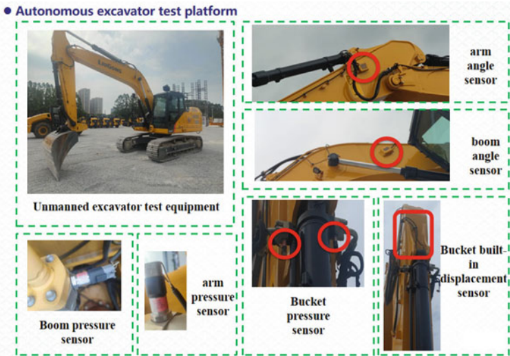
Fig. 6 Autonomous excavator test platform
