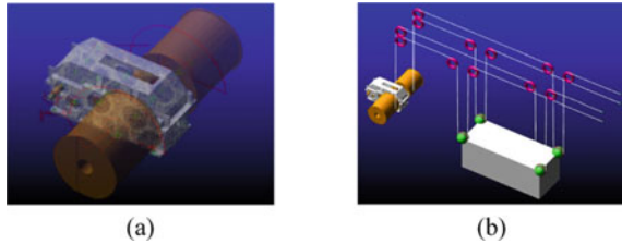
Fig. 7 Model of the driven gear 1 on intermediate shaft 1. a Normal state b Missing tooth state
