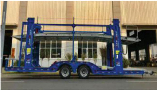
(a) Photos of a central axle trailer
