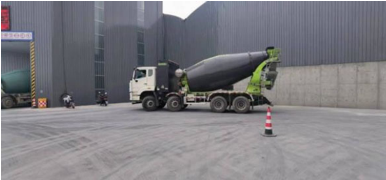
Fig. 5 Our unmanned concrete mixer truck
