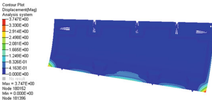
Fig. 7 The deformation contour plot of the APU door
