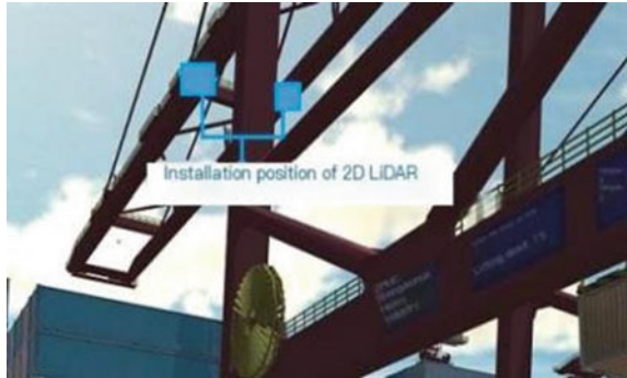
Fig. 3 Installation of virtual LiDAR
