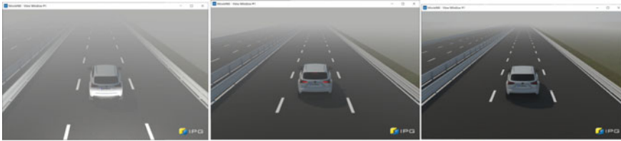
Fig. 5 Test scenario of the front static vehicle under different visibility in foggy days
