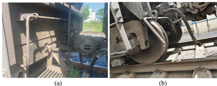
Fig. 2 Original coupler unhook operating handle, a Top acting handle. b Down acting handle
