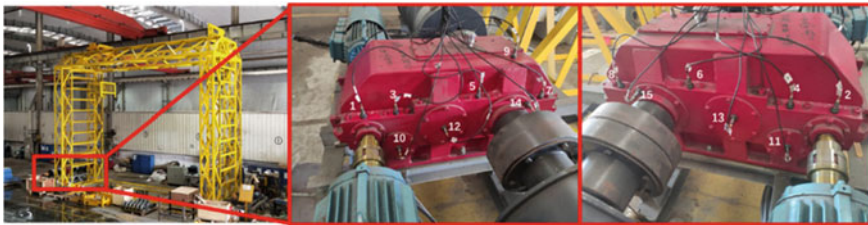
Fig. 10 Scaled test rig of the quay crane gearbox and sensor installation positions (numbers in the picture indicate sensor labels)
