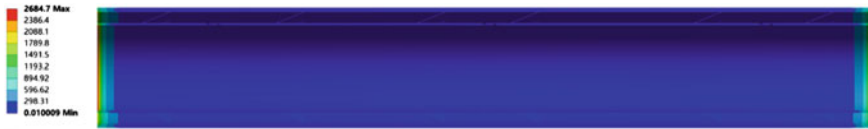
Fig. 5 Stress contour plot of the main pipeline
