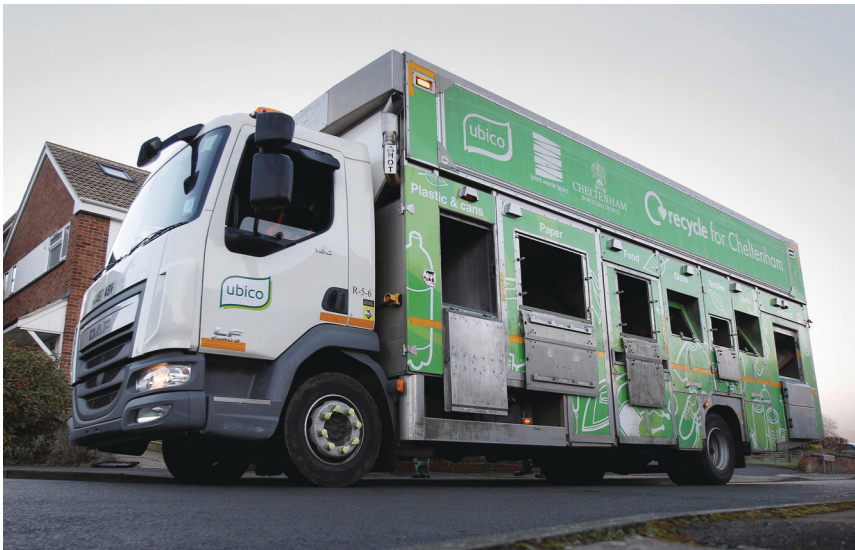
FIGURE 4.2 A source separated collection vehicle. Photograph courtesy of Cheltenham Borough Council/Ubico Ltd.
