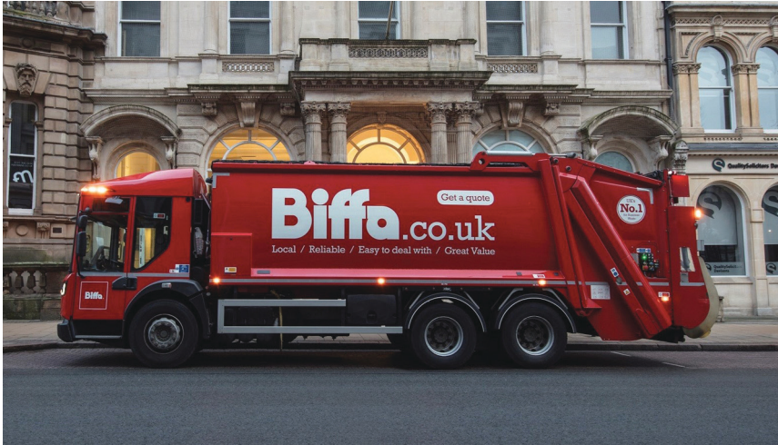
FIGURE 4.1 A standard refuse compactor collection vehicle. Photograph courtesy of Houston PR on behalf of Biffa.
