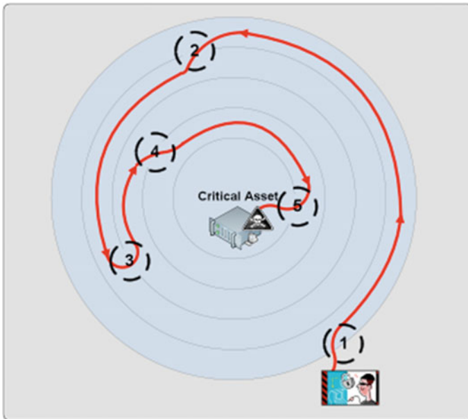
Fig. 7.2 Illustration of defense-in-depth. Multiple barriers must be overcome before the attacker can reach its objective
