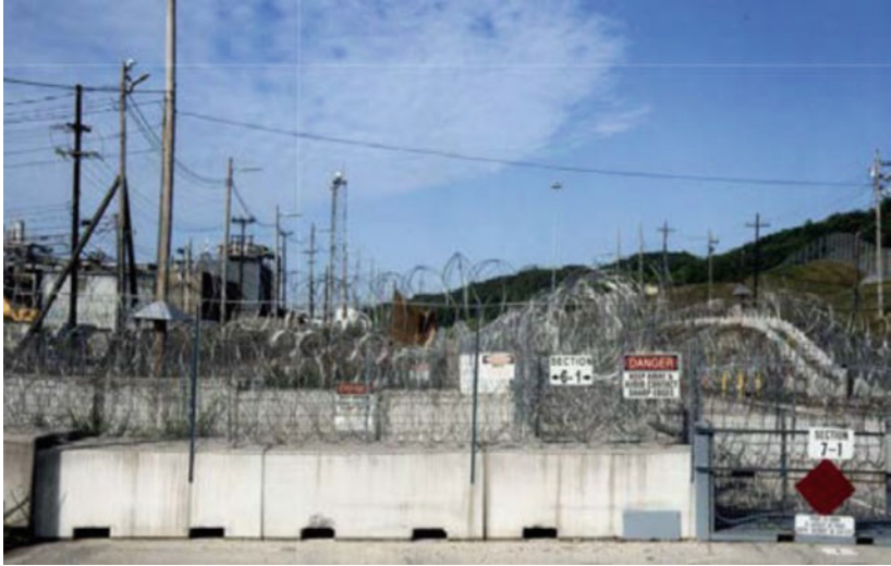
Fig. 3.3 Delay barriers at Y-12 42
