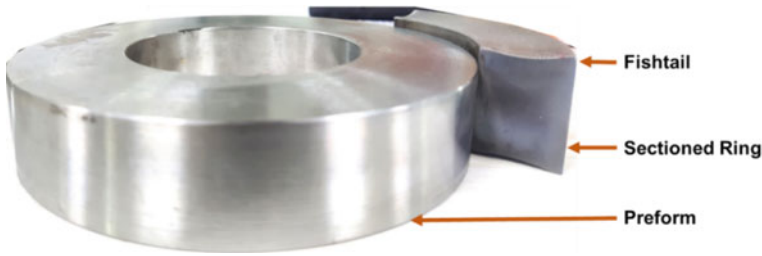
Fig. 10 Photographs of preform and sectioned ring with fishtail defect
