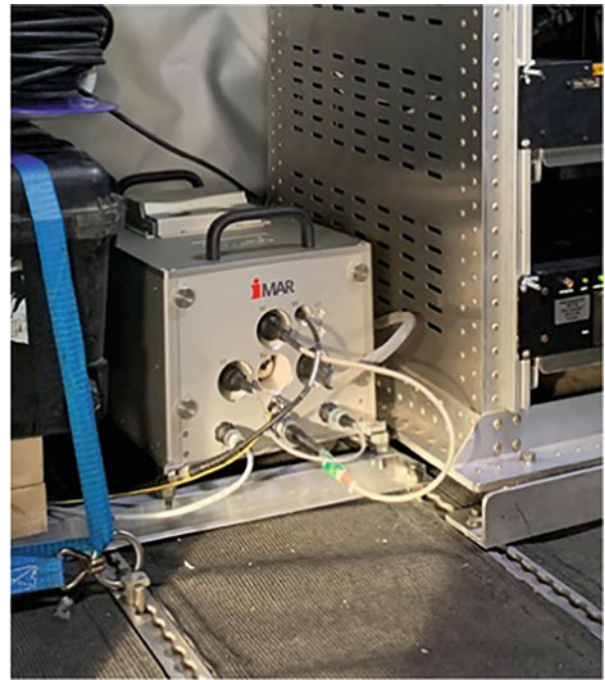
Fig. 1 A strapdown airborne gravimeter on board the aircraft
