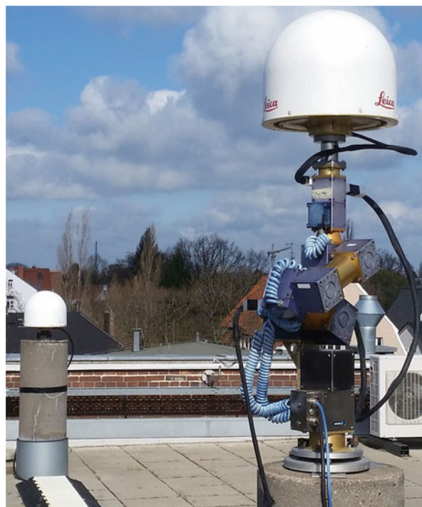
Fig. 1 Antenna calibration setup at IfE with the robot (foreground) and the nearby reference station (background)
