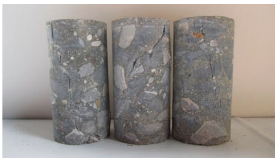
Fig. 2 Failure model of concrete samples subjected to triaxial-seepage coupling conditions
