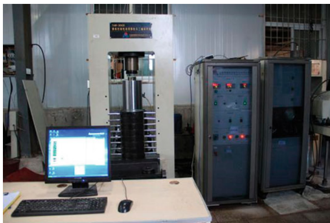
Fig. 1 TAW-3000 electro-7hydraulic servo rock triaxial testing machine
