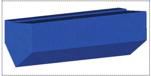
Fig. 4. Finite element mesh of rock wall beam
