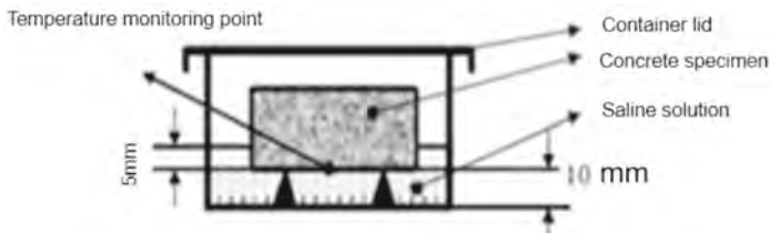
Fig. 1. Schematic diagram and equipment of salt freezing test method
