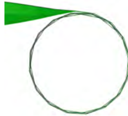
Fig. 9. Untight coiling caused by mesh limit
