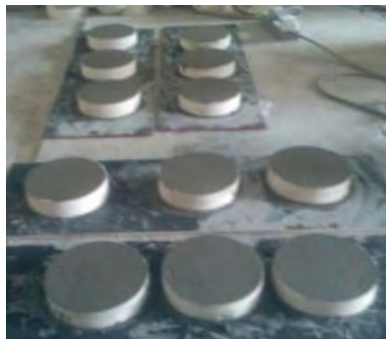
Fig. 2. Forming Method of Salt Frozen Specimens
