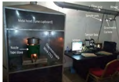
Fig. 8. Laboratory Emissions Monitoring System with the Nozzle type Energy Efficient Cookstove mounted inside the metal hood [14]
