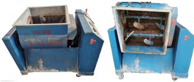
Fig. 2. HJS-60 horizontal double-axis forced mixer.
