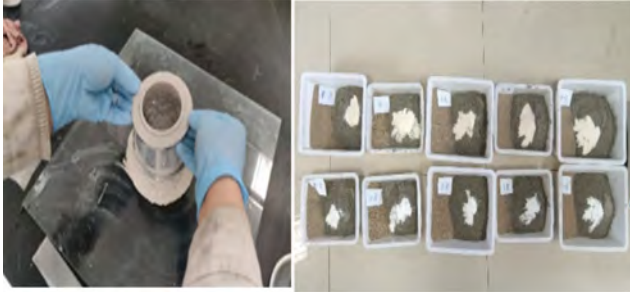
Fig. 1. Variation of fluidity with sand particle size
