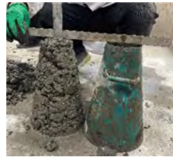
Fig. 3. Slump test process of concrete (4:6)
