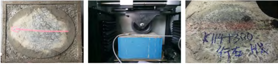
Fig. 1. Accelerated loading test with full thickness of asphalt surface
