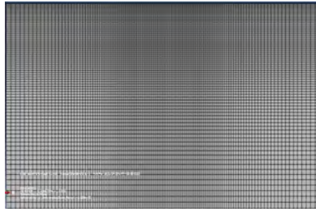
Fig. 2. Pavement structure mesh.
