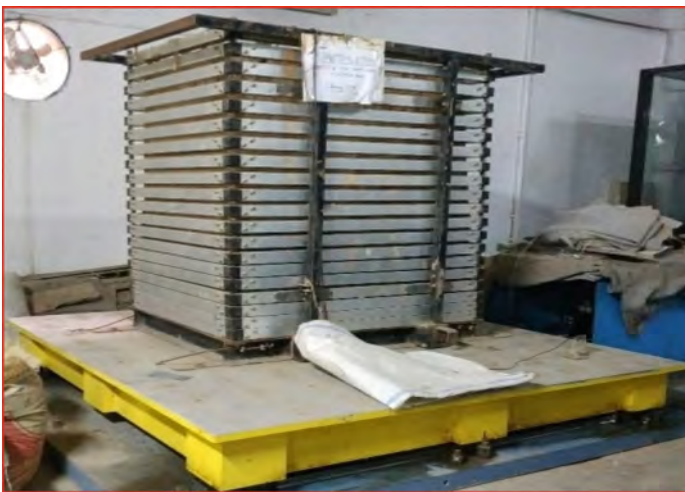
Fig. 1. Seismic analysis of the model embankment
