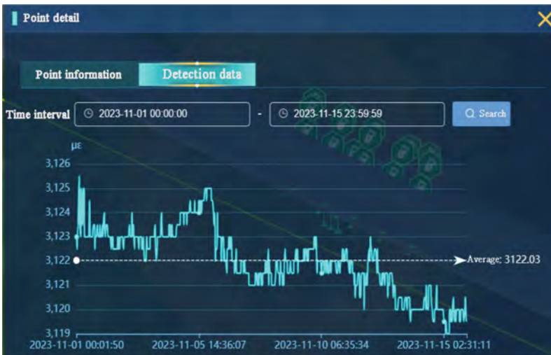
Fig. 8. Tunnel deformation monitoring data map based on tunnel safety multidimensional monitoring and early warning system
