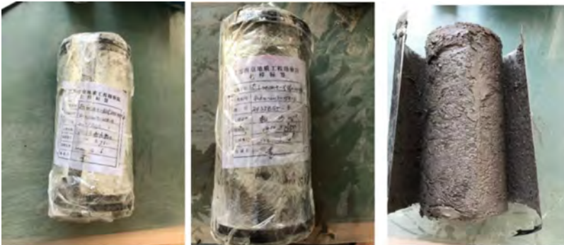
Fig. 1. Thin-wall samples from Nanjing Yangtze River floodplain area.
