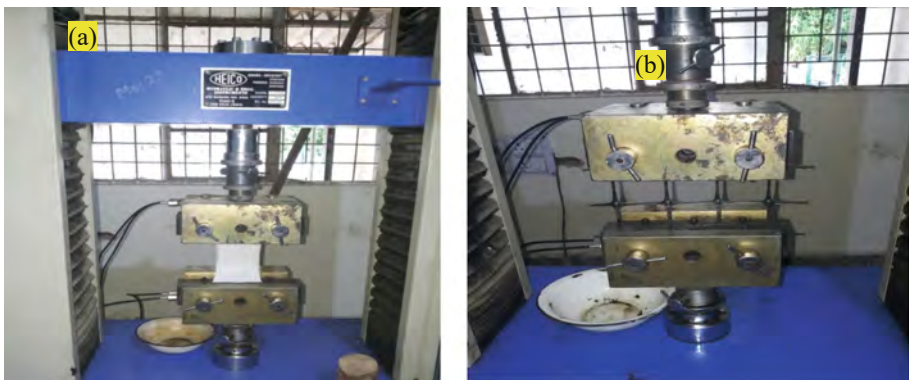
Fig. 2. Geosynthetics creep testing machine, a) Nonwoven geotextile; b) Biaxial geogrid
