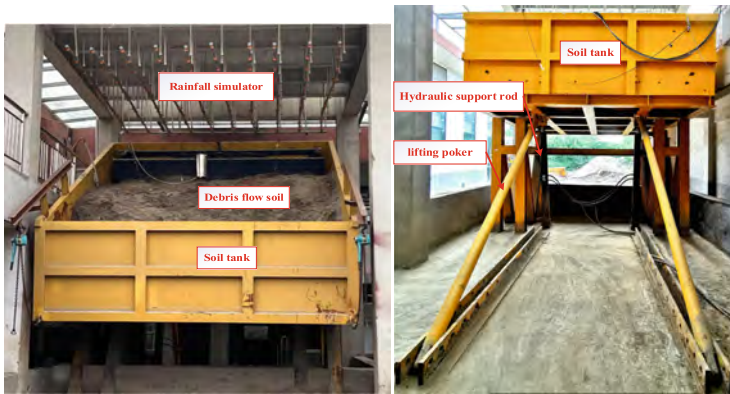
Fig. 1. Slope debris flow simulation experimental platform
