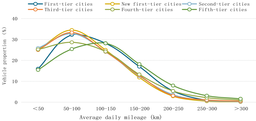
Fig. 4.45 Distribution cars for sharing of different average daily mileages in 2022—by city tier
