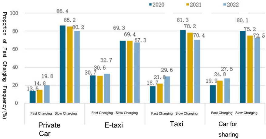
Fig. 8.33 Distribution of average monthly charging frequency of PHEV-passenger cars with different charging methods
