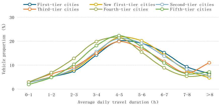
Fig. 4.55 Distribution of logistics vehicles of different average daily travel durations in 2022—by city tier
