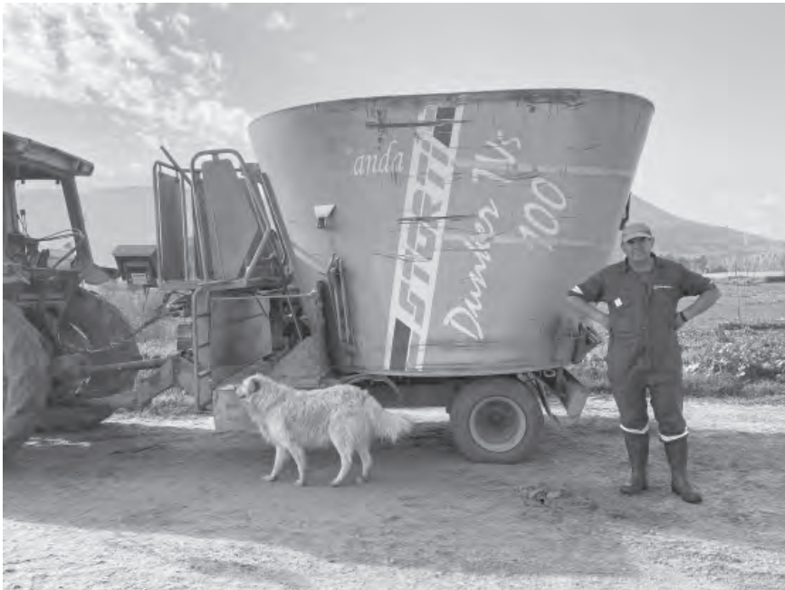
Figure 5.2 Tonino with his Unifeed wagon. It simplifies distribution of feed, reduces labour costs, and allows for controlled and standardized animal feeding. Villamassargia, south-west Sardinia, November 2020.
