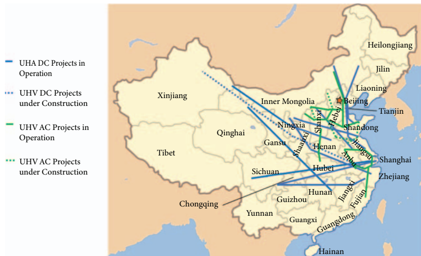
Figure 7.6 China’s UHV-DC and UHV-AC power grid, 2020
