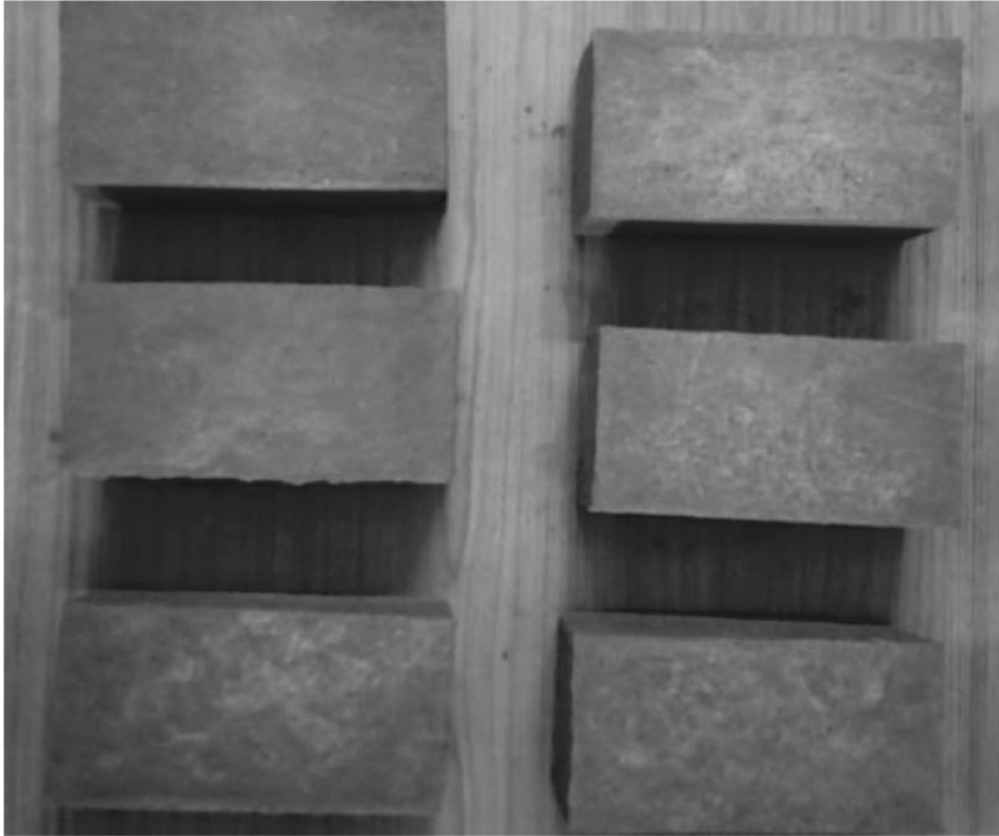
FIGURE 2.11 Agricultural residue-based cement sand bricks.
