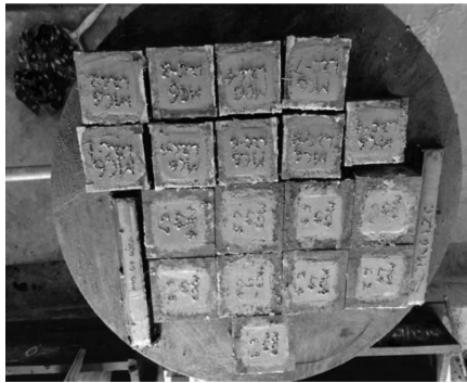
FIGURE 2.8B Cow dung–stabilized mud mortar specimens.
