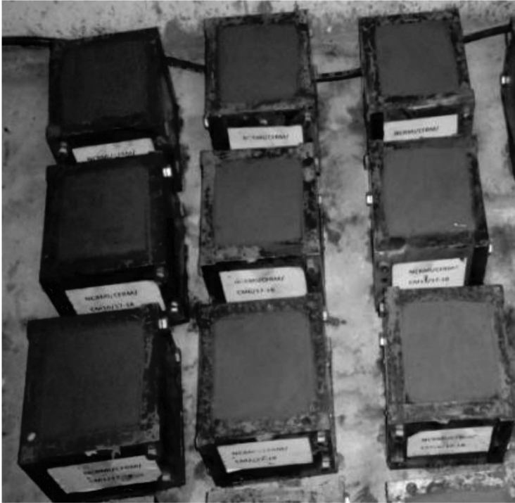
FIGURE 2.7 Agricultural residue-based cement mortar specimens.
