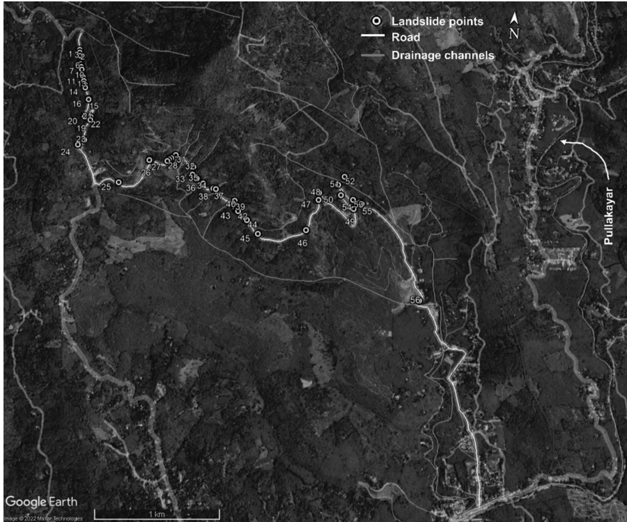
FIGURE 18.2 Landslide inventory data, overlaid on pre-event Google Earth image.
