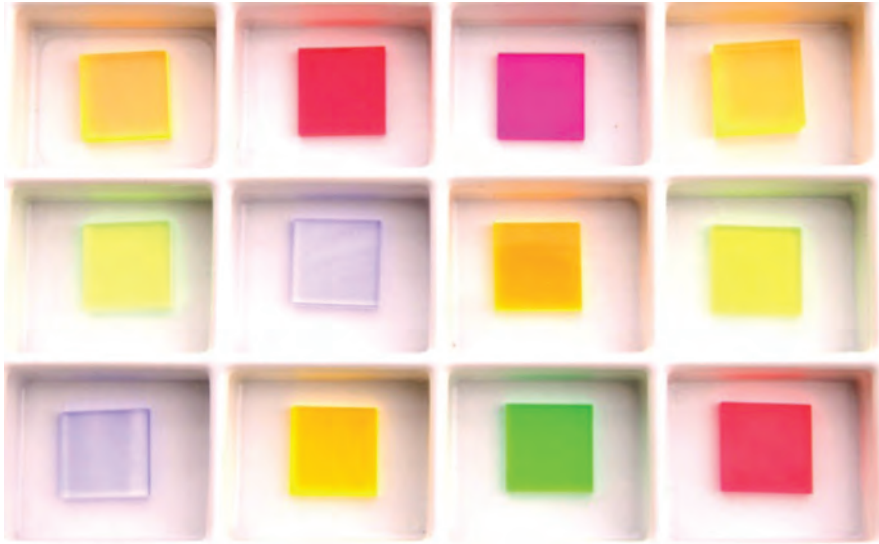
FIGURE 3.5 Possible colors that can be realized with different dyes in luminescent solar concentrator PV applications (From FhG-ISE, 2019.)
