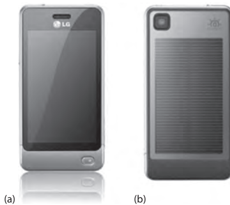
FIGURE 4.14 (a) The GD510 mobile phone by LG. It was introduced as a solar-powered phone, and (b) the phone includes an additional back cover with an embedded solar panel. (Courtesy of LG.)
