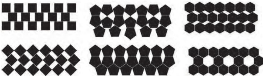
FIGURE DC-2.13 Exploration of basic shapes for the garden fence module with square, rhombus, pentagon, and hexagon. In the prototype, the hexagon was used.
