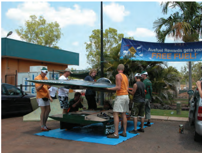
FIGURE DC-4.4 The first solar car of the Solar Team Twente was released in 2005. It had a 9 m 2 GaAs PV array, three wheels, and to step into the car the driver needed support by at least six people. Please notice that 2019 regulations prescribe a maximum of only 2.6 m 2 GaAs solar PV cells.
