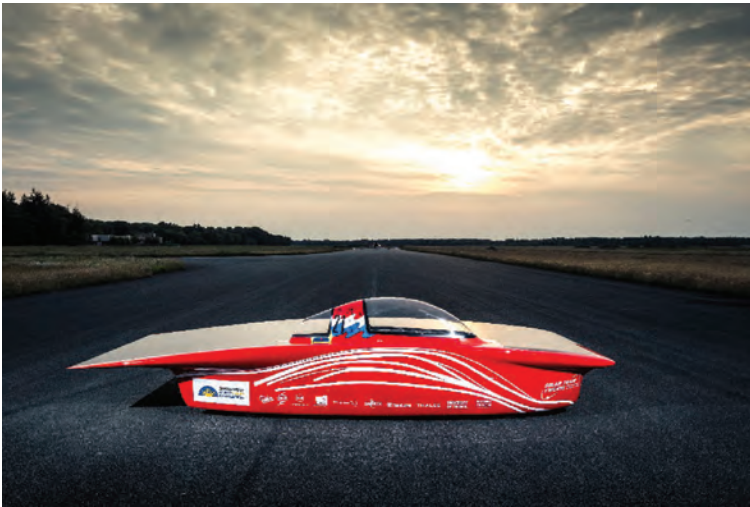
FIGURE DC-4.12 The solar panel of the RED One (2015) has barely any curve left to decrease drag.
