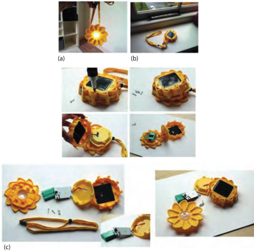
FIGURE 6.17 (a) Little Sun light is turned on; (b) Little Sun PV-powered light is placed near the windowsill for charging; and (c) disassembling the PV product during the field trial. All parts of the product are visible, including plastic components (casing), cables, screws, and PV cell.
