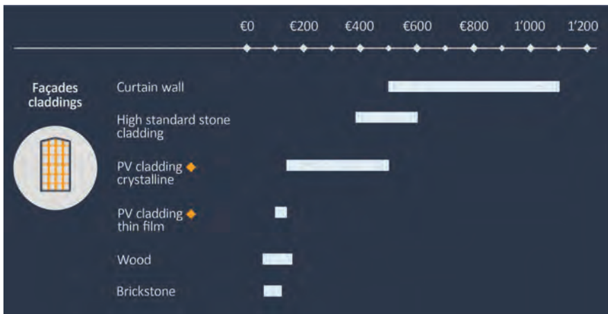
FIGURE 5.28 PV costs compared to other cladding materials used in the built environment as façade cladding materials. (From Zanetti, I. et al., Building integrated photovoltaics: Product overview for solar building skins, Eindhoven (NL) & Lugano (CH), www.seac.cc, 2017.)
