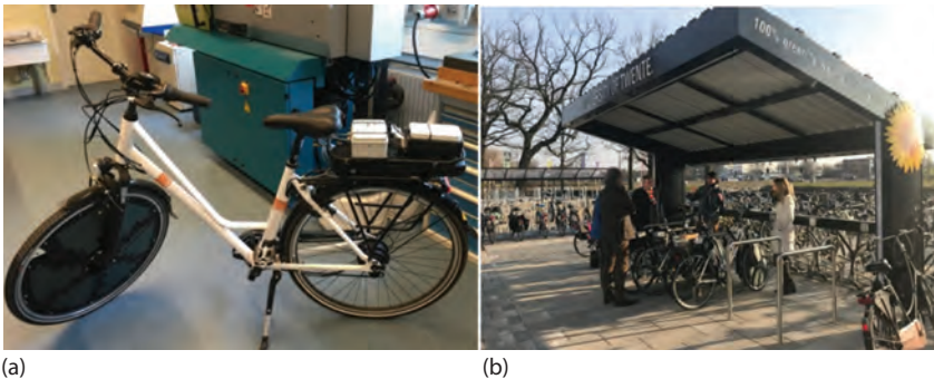
FIGURE DC-6.1 (a) Solar e-bike, and (b) PV-powered charging station in UT campus.
