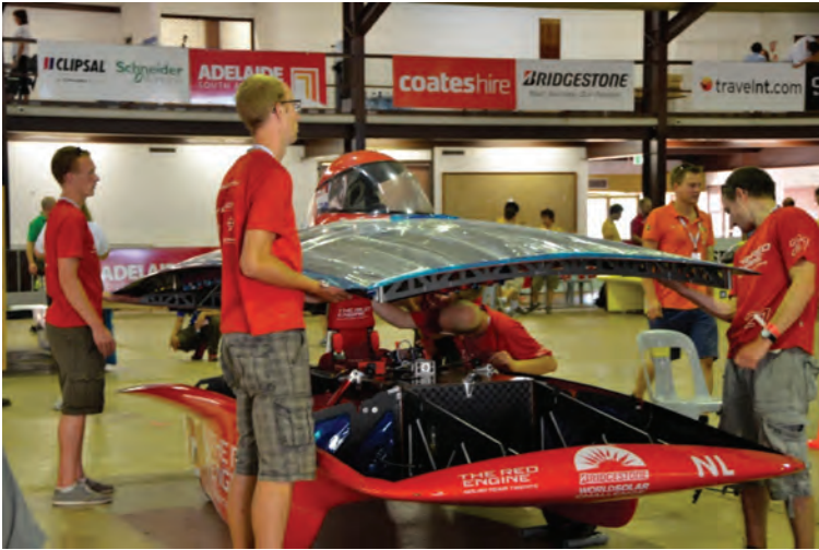
FIGURE DC-4.5 In 2013, the Solar Team Twente participated in the BWSC with the RED Engine, which has a 6 m 2 silicon PV array, and it takes “just” four people to close the PV panel. Please notice that this was the first solar car of the Solar Team Twente with four wheels.
