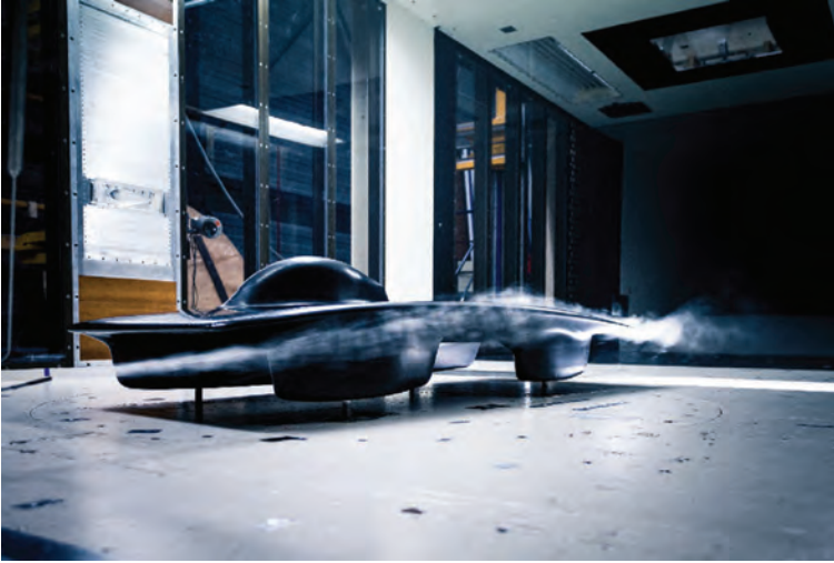
FIGURE DC-4.8 A scale model of the RED One was tested in a wind tunnel. The models used to design the car were compared to the airflow simulated in the tunnel.
