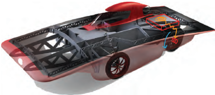
FIGURE DC-4.10 A schematic overview of the energy flow from the battery to the motor.
