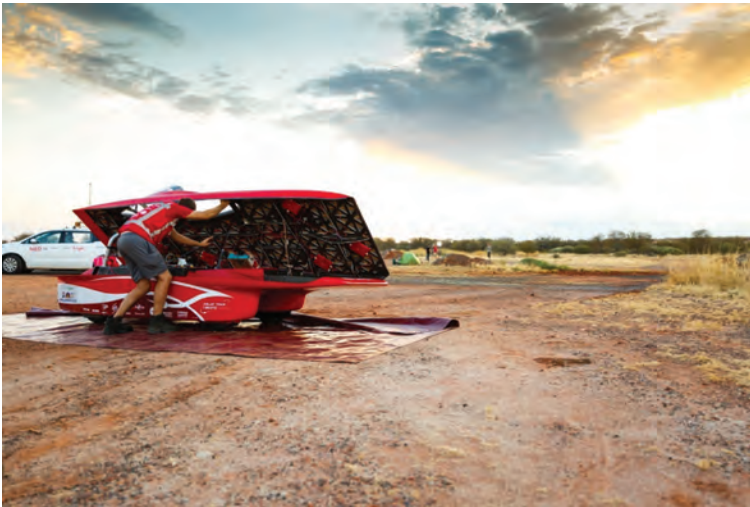
FIGURE DC-4.6 RED Shift, the 2017 car, was a lot smaller than the previous cars, having a 4 m 2 silicon solar panel. This was also the first solar racing car in which the driver was able to enter and close the panel without any help of team members.
