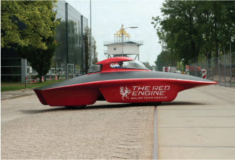
FIGURE DC-4.11 The RED Engine (2013) clearly has a curved PV panel.
