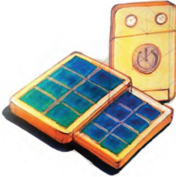
FIGURE 6.16 One of the proposed redesigns of the Waka Waka lamp, according to lead-users suggestions; the solar-panel area is extended.
