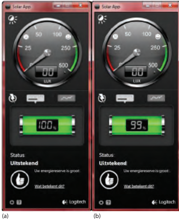
FIGURE 6.23 The solar application of the Logitech solar keyboard, showing the light brightness and the charging status of the battery (a) before starting the test, and (b) after 4 days of use.
