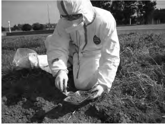
Figure 3.3 Professor Anzai, in anti-contamination suit, gathering soil samples from a paddy field about 7 kilometres from the Fukushima nuclear power plant in April 2011. The soil was found to be extremely contaminated with radioactive substances such as Iodine 131, Cesium 134 and Cesium 137. Special exhibit on Radioactivity and the Future of Humanity , Kyoto Museum for World Peace. Credit: Anzai Science and Peace Office, Fukushima Project for a Safer Future.
