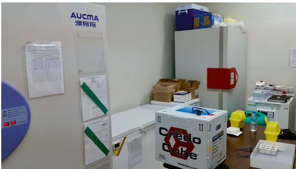
Fig. 5 A mixture of freezer types used at a study storage depot site in Freetown, Sierra Leone, including upright, chest, and passive transport containers. (Photo: Matthew Kirchoff)
