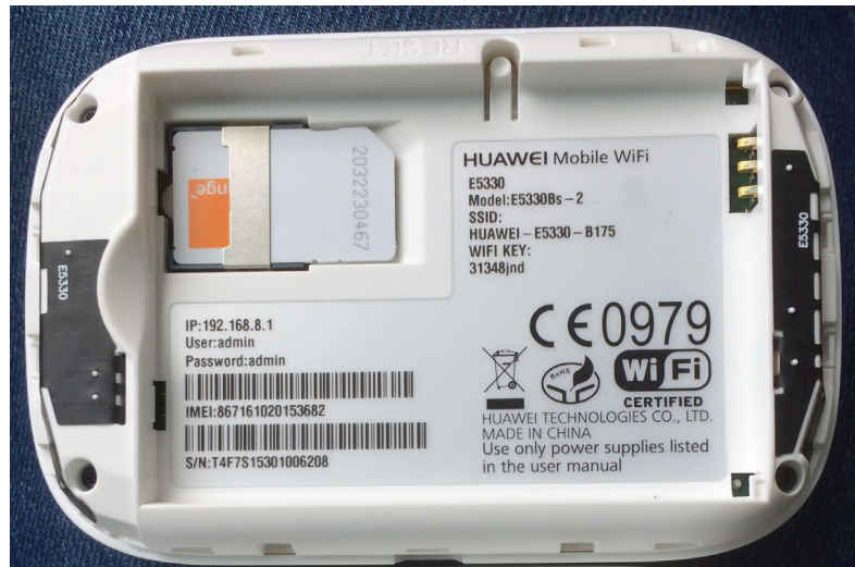
Fig. 6 A mobile hot spot device and SIM card used as an Internet backup device for real-time electronic temperature monitoring. (Photo: Matthew Kirchoff)
