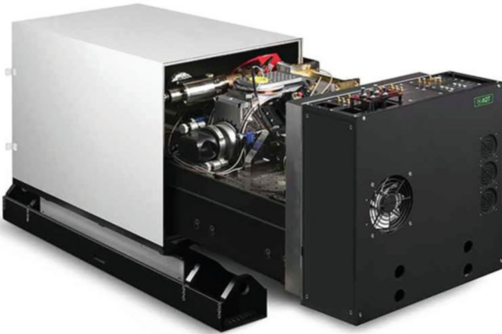
Fig. 7 This configuration of the PINE setup is ready to be mounted into a standard 19" rack with easy access by mounting it on sliding rails which act as a drawer that can be pulled out of the rack. Additionally, it features a vibration isolation stage, a scientific camera for imaging purposes, and an electromagnetic shielding structure
