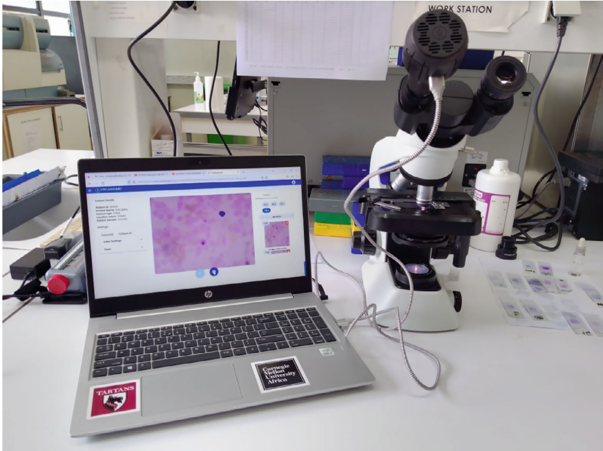
Fig. 1 Camera mounted on microscope at RBC to collect digital images of microscopic slides
