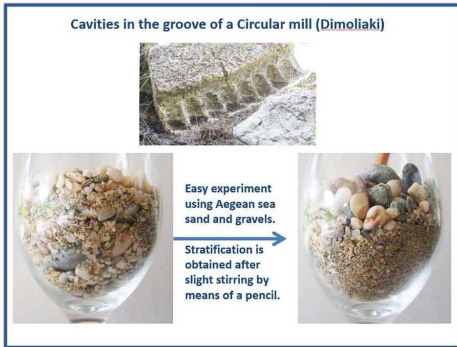
Figure 8. Stratification inside the cavities of the groove in circular mills
