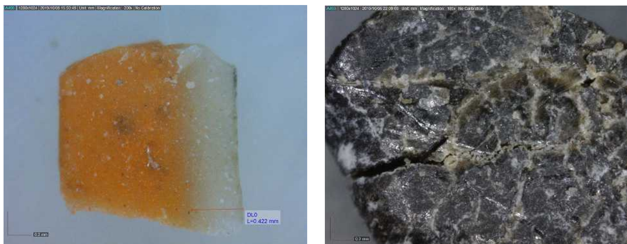
Figure 1. (a) Side view and measurement of the alteration zone on sample A small fragment and (b) Detail of the micro-cracking on the external surface of sample B.
