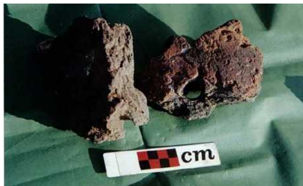
Figure 3. Sideri (Kythnos): Metallurgical furnace fragments with perforations (Bassiakos-Philaniotou 2007).
