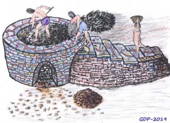
Figure 6. Schematic representation of the roasting furnace, while charging with galena ore from the mouth.
