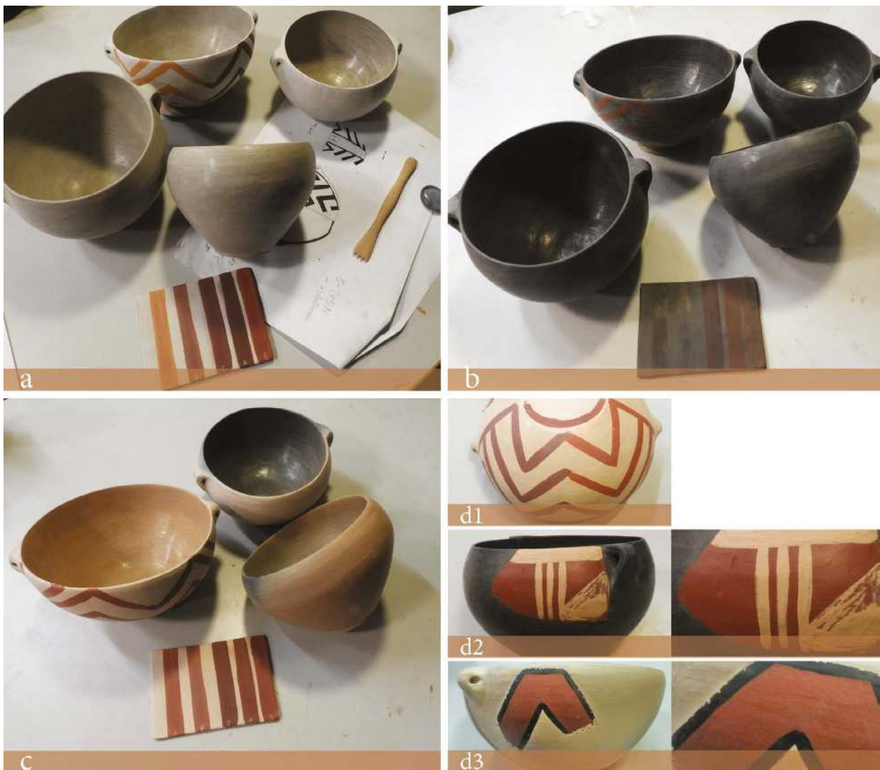
Figure 8. (a) Hand built and polished bowls before firing. The two bowls on top middle and right are coated with a light coloured slip, while one of them bears a painted decoration with Fe-oxides; (b) the same bowls after reducing firing at 600°C; (c) refiring at 700°C in mixed/oxidising atmosphere led to clear colours - see d1, case of the sherd NGAL-2 in Figure 1a - or to cloudy appearance depending on the placing of the pots; (d) application of red 'crust' with a light coloured clay using an organic binder (case of sherd NGAL-8 in Figure 1b), and application of red and black pigments on a fired light coloured slip (case of the sherd NGAL-3 in Figure 1c).
