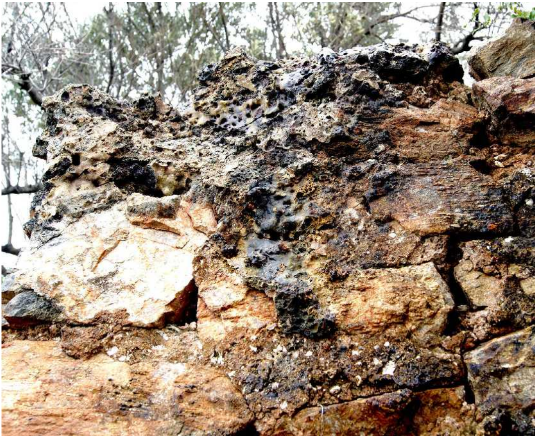
Figure 5. Slag foam coming from the most fusible components of the galena ore remain attached on the wall on top, near the furnace mouth.
