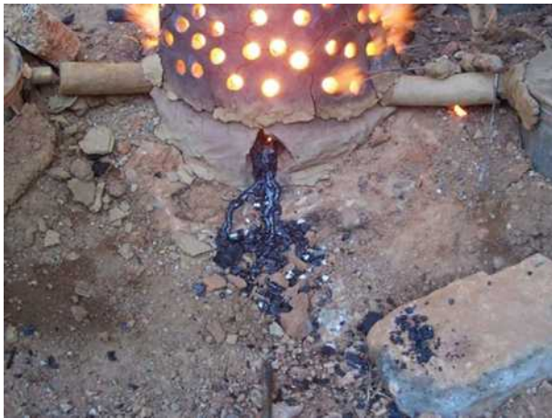
Figure 9. Smelting slag with low viscosity allowing to flow outside the furnace (Courtesy Dr Y. Bassiakos).
