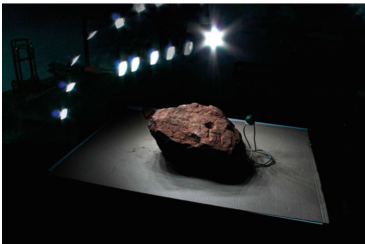
Fig. 5 Frame from an H-RTI session recording the Nessglyph
