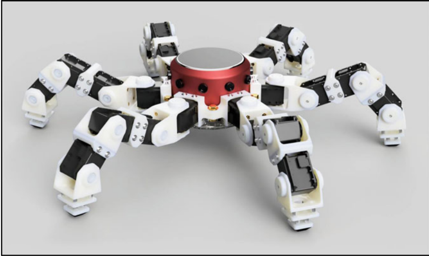
Image 5 Rendering of a Hexapod Robot. Modelled in Fusion 360 parametric 3D modelling system from Autodesk. (Derivative of 'Anansi Hexapod Robot' by Bryce Cronin/CC BY 4.0. www.cronin.cloud/hexapod )
