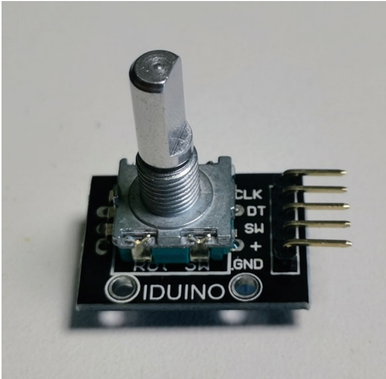
Fig. 7.9 A popular hobby rotary incremental encoder with two outputs (quadrature encoder)
