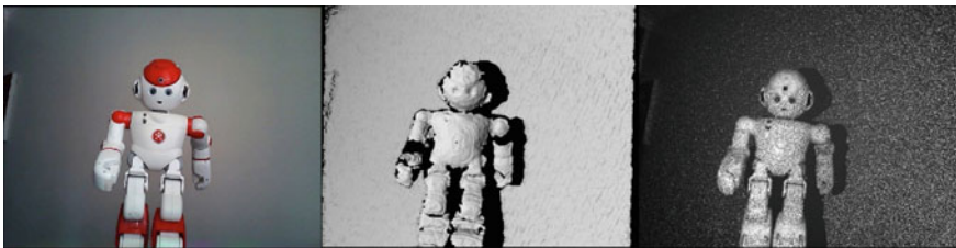
Fig. 7.7 A view from an RGB-D camera (from left to right—RGB image, depth image, IR image showing the projected pattern)
