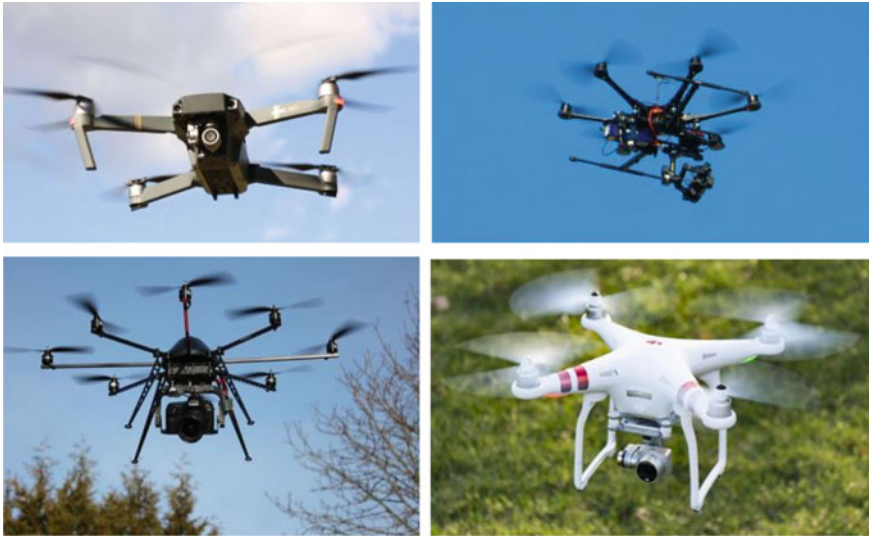
Fig. 8.13 Different types of multicopper (clockwise from top left—A quadrotor—DJI MAVIC PRO, A hexacopter—Custom built model, DJI Phantom Model and An octocopter—Custom built model)
