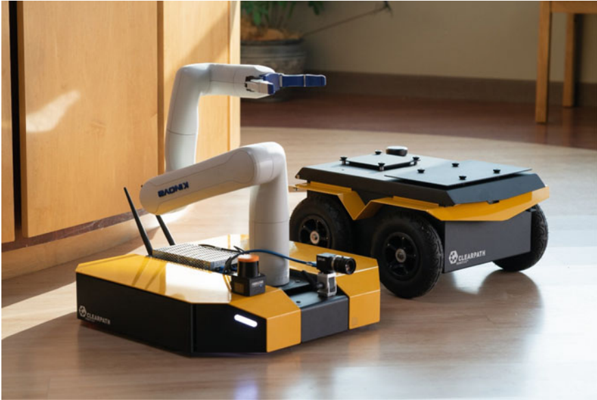
Fig. 8.1 A Kinova Gen3 lite robot arm mounted on a Clearpath Dingo Indoor mobile robotic platform (left) alongside a Jackal Unmanned Ground Vehicle used for outdoor navigation. (right) (Credits Clearpath/Kinova)
