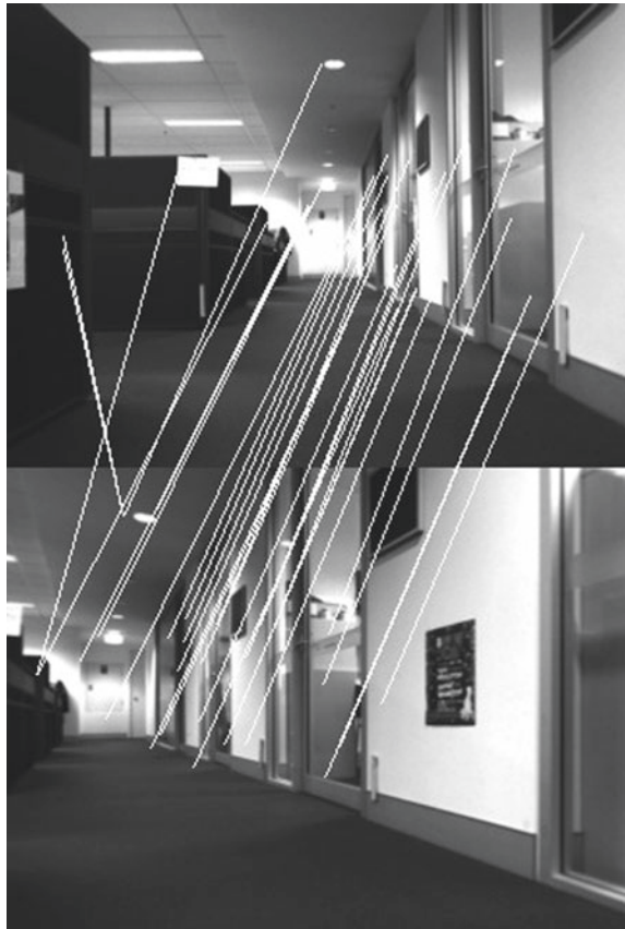
Fig. 9.7 A vision algorithm is used to detect salient features in the environment. The top and bottom images show two views of the same environment captured at two different time intervals of the robot's journey. The lines indicate matched features between the two images (data association). Can you spot any instances of failed data association?
