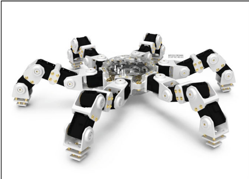
Image 15 UC Hexapod Robot 3D CAD model. Built in Fusion 360 CAD software. (Bryce Cronin/CC BY-NC-ND 4.0. www.cronin.cloud/hexapod )
