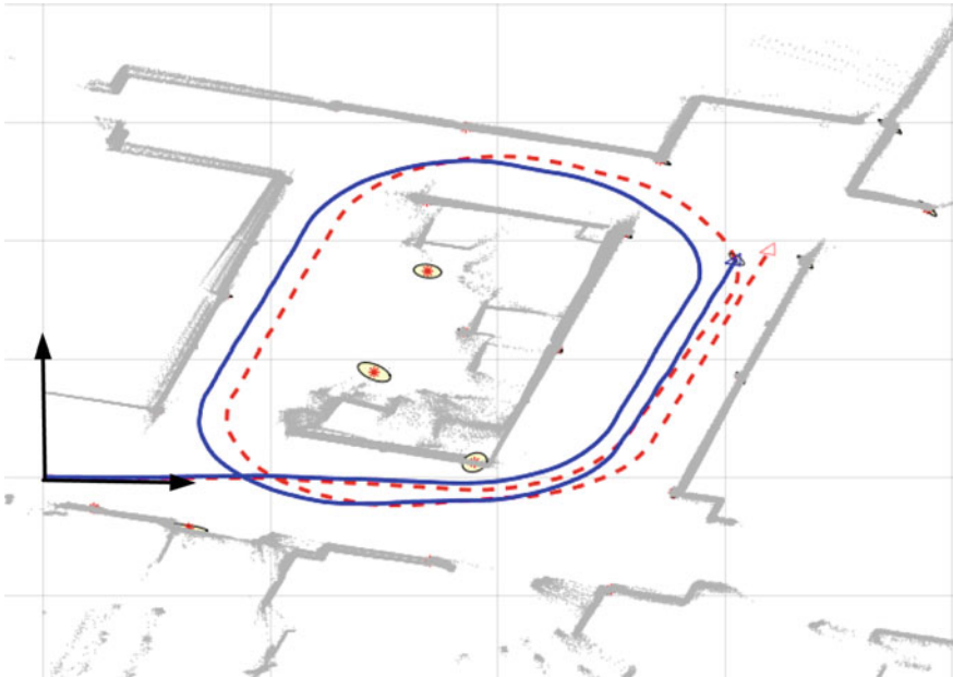
Fig. 9.11 An implementation of the EKF-based localisation algorithm. The solid blue line indicates the EKF estimate of the robot path. The red dotted line is odometry. The * denotes the locations of the surveyed beacons
