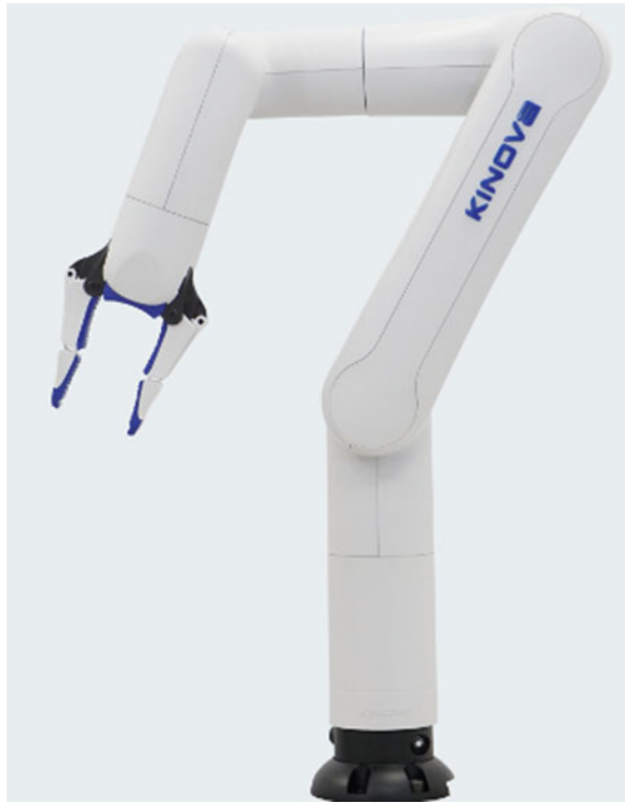
Fig. 10.1 Kinova Gen3 lite, a serial 6-DoF robotic manipulator
