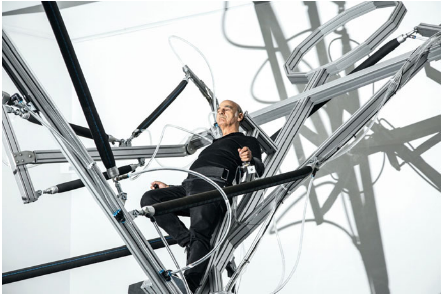
Fig. 7.12 Pneumatic rubber muscles used in animating this giant robotic structure during a performance by the artist, Stelarc (Reclining StickMan, 2020 Adelaide Biennial of Australian Art: Monster Theatres, Photographer—Saul Steed, Stelarc)
