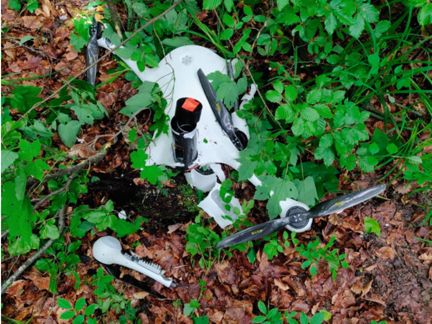
Fig. 16.1 Matternet (2021) drone which crashed in a wooded area of Switzerland near a kindergarten. The emergency parachute had been deployed, but the chord connecting it to the drone was cut allowing the 12 kg drone to freefall to the ground. Image used with permission, from SUST (2019)
