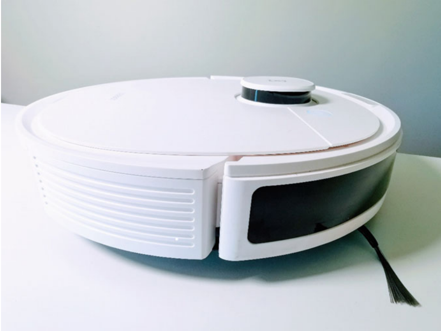
Fig. 7.10 A modern vacuum cleaning robot integrates many sensors. On the top is a time-of-flight laser scanner. The front bumper includes several tactile sensors to detect any frontal collisions. What other sensors do you think this robot may have?
