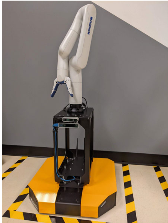
Fig. 18.8 Mobile manipulator platform in its parking space
