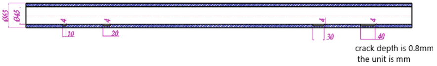
Fig. 14 Pipes of different length crack
