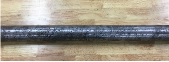
Fig. 10 Pipeline with the cracks in the range of 0^{\circ} – 90^{\circ} orientation
