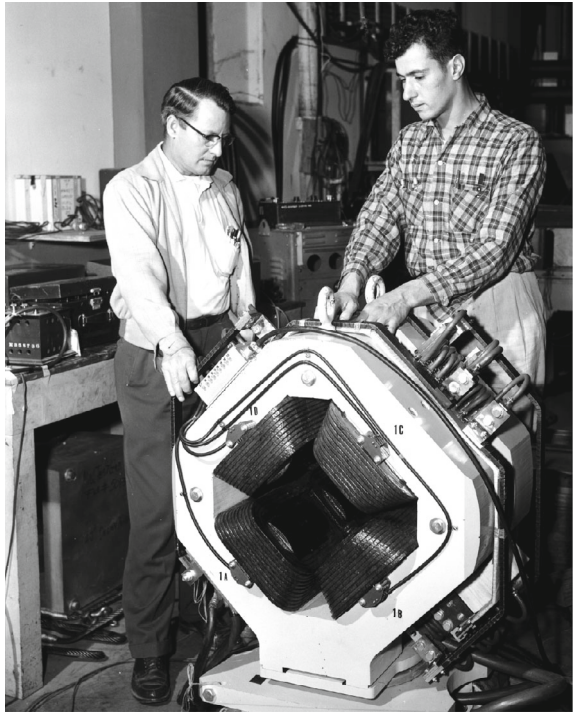
Fig. 9.3 SATURNE2 strong focusing 3 GeV synchrotron at Saclay [5], successor in the late 1970s of SATURNE1 weak focusing synchrotron (Fig. 8.1). It was the first strong focusing synchrotron to accelerate polarized ion beams
