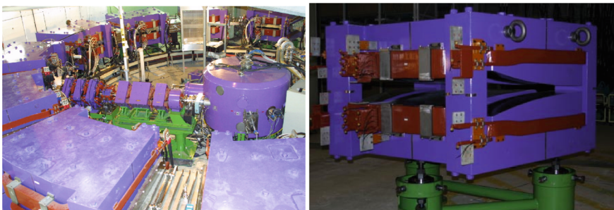
Fig. 10.6 Left: KEK 150 MeV 12-cell scaling FFAG ring, and its cyclotron injector [10]. Right: Its lattice cell magnet, a DFD dipole triplet. The gap shape follows Eq. 10.6 so ensuring the scaling field law (Eq. 10.5) [23]
