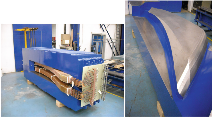
Fig. 10.3 Full scale prototype (left), and pole (right), of the spiral sector dipole of a proton FFAG designed for proton-therapy use [13]
