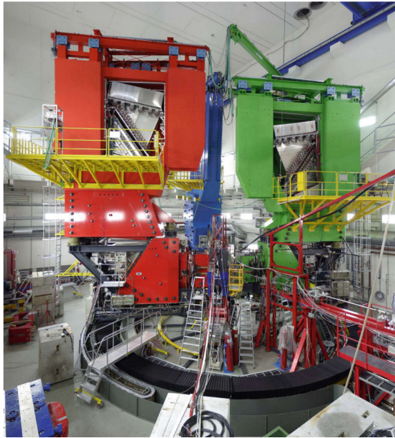
Fig. 13.3 Magnetic spectrometers at GANIL. Left: SPEG, in operation since 1985, shown here with its upstream analysis section. SPEG was designed using zgoubi, by Birien and Saby Valero [4], early developers of the code. Right: LISE [5], used for atomic physics and isotope studies
