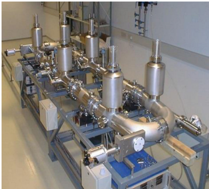
Fig. 2.7 Elisa in Aarhus, a 25 keV, 7.6 m circumference racetrack for molecular and atomic physics [10]. Its lattice combines spherical deflectors, plane deflectors and quadrupoles
