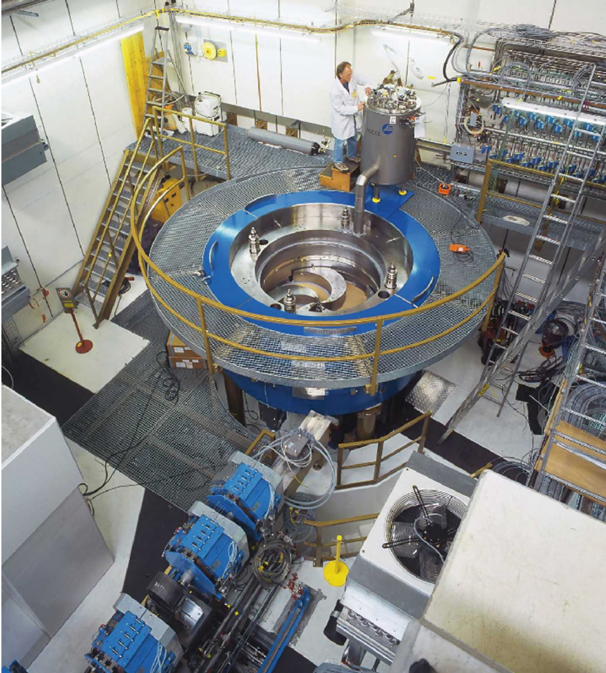
Fig. 4.1 COMET protontherapy cyclotron at PSI. A 250 MeV, 500 nA, 4-sector isochronous AVF cyclotron. The spiral poles enhance axial focusing. A 3 m diameter superconducting coil provides the dipole field [2]
