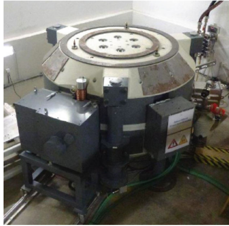
Fig. 7.2 The 230 MeV superconducting S2C2 [7], a 1 kHz repetition rate compact synchrocyclotron for protontherapy. Parameters: RF frequency 60–90 MHz; magnetic field 5 T; overall diameter 2.5 m; weight 50 Ton
