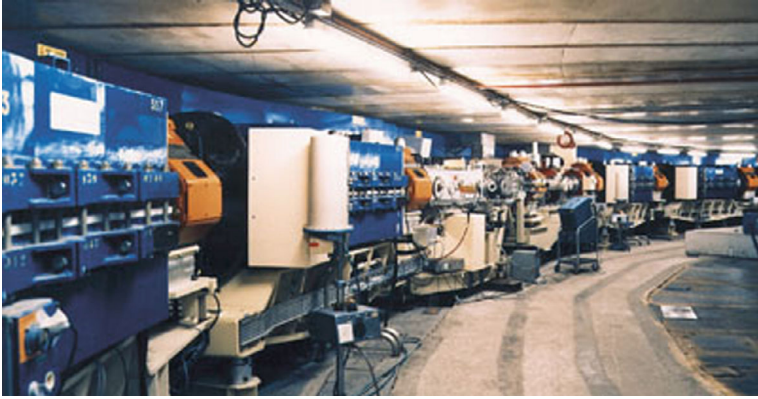
Fig. 9.3 SATURNE2 strong focusing 3 GeV synchrotron at Saclay [5], successor in the late 1970s of SATURNE1 weak focusing synchrotron (Fig. 8.1). It was the first strong focusing synchrotron to accelerate polarized ion beams
