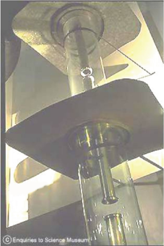
Fig. 2.1 A similar tube cascade to the early 1930s Cockcroft-Walton experiment eponymous acceleration system: Fermilab’s 750 keV H^- injector [2]
