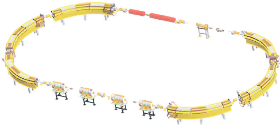
Fig. 9.6 The ion rapid cycling medical synchrotron (iRCMS) [9], an ion beam RCS for the treatment of cancer tumors
