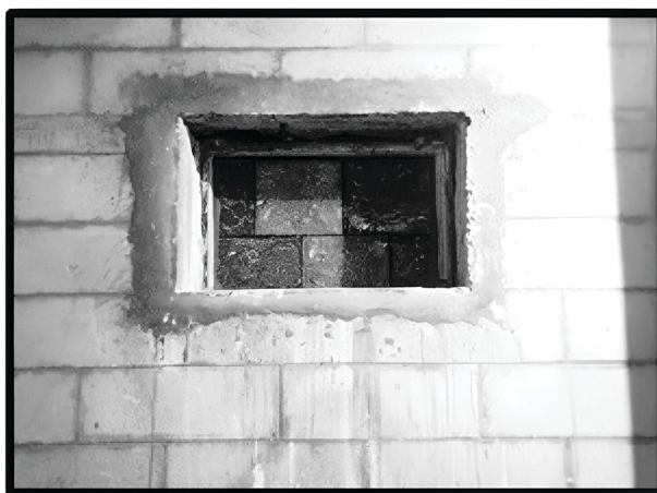
FIGURE 7.9 Sound transmission loss measurement in the reverberation chamber.
