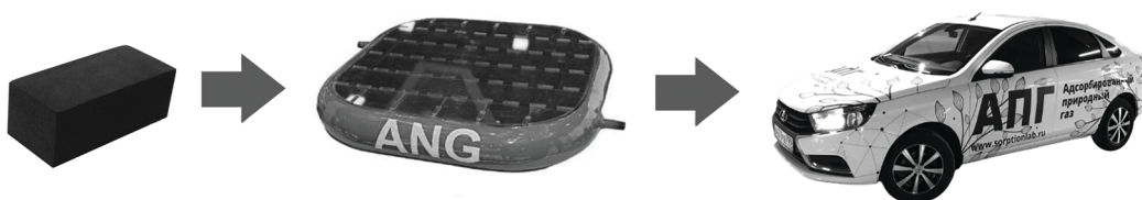
FIGURE 6.9 Functionalized monolith carbon adsorbent M-C-1 that fills the prototype of the ANG system for the gas-powered vehicle for a car.
