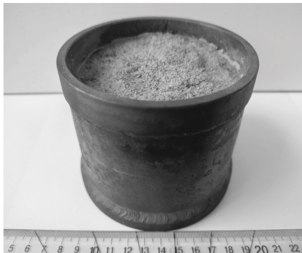
FIGURE 12.1 Overall view of ceramic matrix containing HLW imitators in a steel container.
