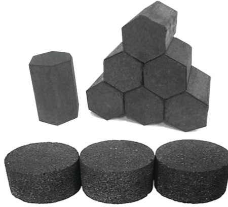
FIGURE 6.1 Monolith blocks of C-1 carbon adsorbent prepared by compacting with the polymer binder under the pressure of 30 MPa.
