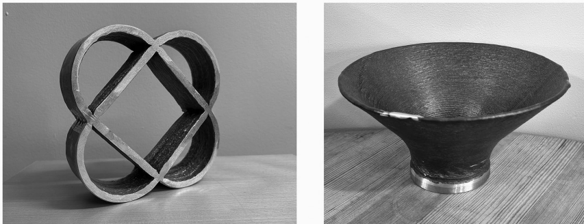
Figure 10.7 Structures with overhang and intersections built using WAAM.
