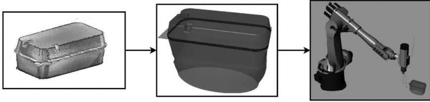
Figure 11.5 Steps from the tool trajectory generation algorithm. The scan is registered to create a joined point cloud. This scan is used to create a 3D mesh representation of the workpiece and the burr region is identified. The generated mesh and the labeled burr region were used to generate the tool trajectory. The figure is inspired from Onstein et al., from which copyright is obtained [20].
