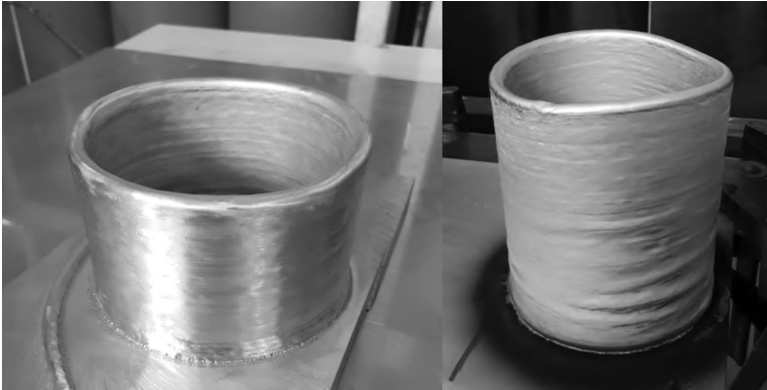
Figure 11.17 Comparison of cylinders created using fixed orientation, left image, and using the field-of-view task, right image. The images appeared in Evjemo et al. [53], an open-access article under the CC BY-NC-ND license. We thank the authors for accepting the re-use in this chapter.
